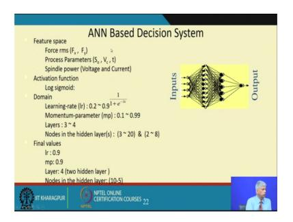
So, this is the artificial neural network based decision system which we used. So, the parameters where the forces process parameters speed depth of cut machining time spindle power and then certain log sigma del activation function was used in the ANN model and we were our three four players and every nodes in the hidden layers with played around with all those these may couple of students got there and a masters degree out of it believe one of them got an award out of and this is work.
