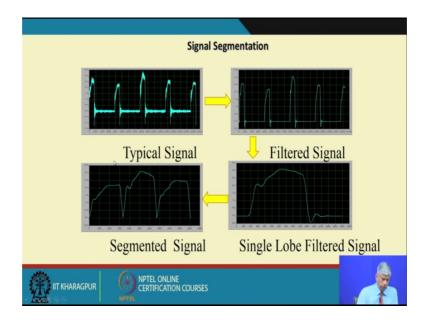
So, a typical signal as you can see, it has lot of noise over it. So, we did a low pass filtering and then this is the filtered signal, ok, I am in where we have remove the high higher frequency effects and then you will see this, there is no information.
