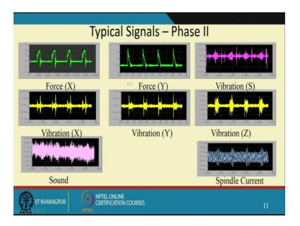
So, for different machining conditions we captured all the machine parameters and this is the typical signals. So, you have the force signals the vibration signals spindle vibrations, the machine vibration signals the noise signals which I have told us sound and the spindle current, etcetera. So, once we get the signals, you will recall, I had told you in signal domain analysis whenever we have a signal we will extract the features.
