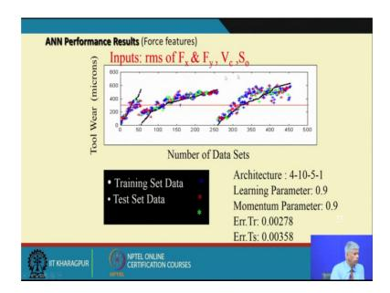
So, the tool were for different data sets, when the tool were with the different data sets when we took the training data set and the test data set.
