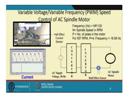
So, just a give you an view now you all know about motor current now. So, this is this Hall Effect sensor used because this had a very well frequency dry if ok. So, you put an hall effect sensor where in we could change the speed of the motor spindle motor by changing by frequency and you will see for no load case when there is nothing being machine the current is nicely a sign wave and I have a single component ok.
