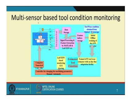
So, this was a multi sensor based tool condition monitoring work where within, I have this machine here and the idea behind this is why are you doing this tool condition monitoring because what you know. So, happened if the tools condition is very blunt it is not sharp I may be damaging the tool or damaging the work piece ok.
