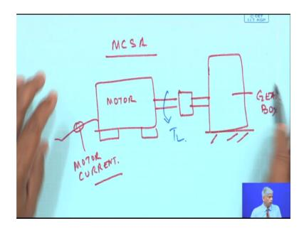
So, just give us a clue why not we use MCSA to find out falls in mechanical system being driven by electrical motors. So, then and now we studied gearbox and so on which I had discussed earlier ok, but this research was our origin of finding out MCSA ok. So, any load torque which comes because of a defect and in this particular case it is because we are missing steel. So, we have current force vibration and then we have other features.
