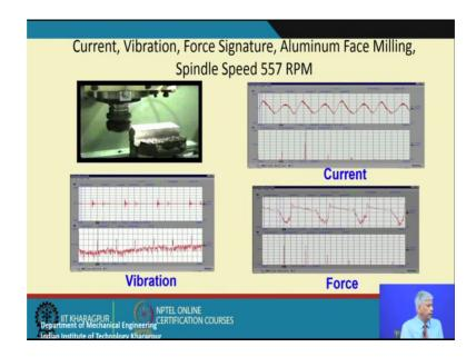
And of course, I was telling you this machining operation we monitor the current by the hall effect sensor we monitor the spindle vibrations and we measured also the force by putting this work piece on a cutting tool force dynamometer ok. So, every time the single tooth comes in contact with the surface there is a force and comes out.
