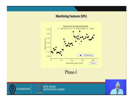
Feature some pressure level some of the parameters from this experiment we were not happy with SPL and acoustic emission for two reasons SPL was contamination with background noise in shop floor, it becomes difficult to monitor the background noise in a shop floor and what influence the machining has rather even acoustic emission there was issues with SNR.
