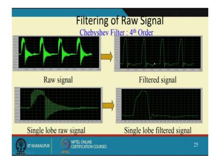
So, this is the output of a filtered signal the raw signal ok, filtered lobe signal lobe raw signal filtered lobe signal.
