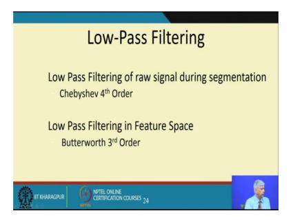
So, there is a good amount of correlation between the training and the testing we tried this parameters and of course, for the low pass filtering by used a Chebyshev fourth order filter and in feature space we used a Butterworth third order filter ok.
