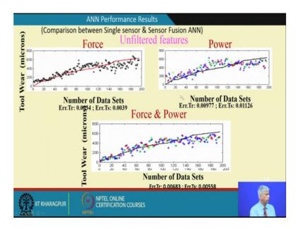
So, we could predict the tool wear within the data sets and there is good amount of predictions with force power and so on ok. .
