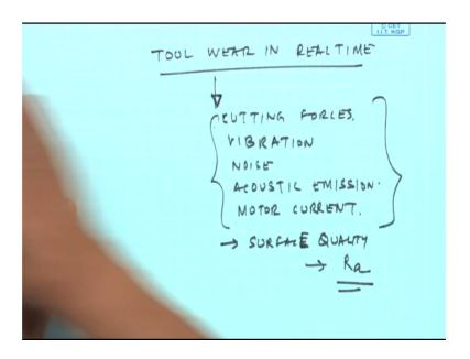
So, to optimal optimally utilize the tool we need to know it is tool wear in real time ok. So, what is this tool wear going to do tool wear is going to generate with the tool is blunt it, it will generate more cutting forces cutting forces would increase we can very related a to a blunt knife and a sharp knife.
