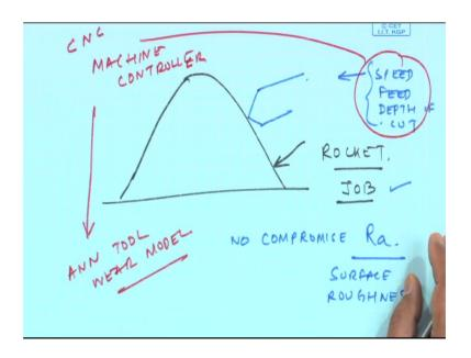
Sometimes you know large machining one of them machining a dome of a rocket. So, it is one of a kind job, I do not want my blunt cutting tool to damage these surface. So, in such a condition what you can do, you can reduce the speed feed depth of cut. So, that at least the job gets done complete the job at lower rates, but nevertheless no compromise on the surface roughness.
