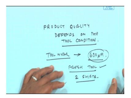
My product quality is going to deteriorate depends on the tool condition ok. So, the flank wear of tool wear which we will discuss usually beyond 600 microns. So, you are manufacturing specialist will say is time for the tool is blunt and it is to be replaced. So,
