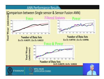
So, you can refer to that paper. So, now, what happens once I measure the force and power out of this machine I can very easily say well that is your tool were and at 600 microns in it you replace the tool. So, this is the power of such ANN.
