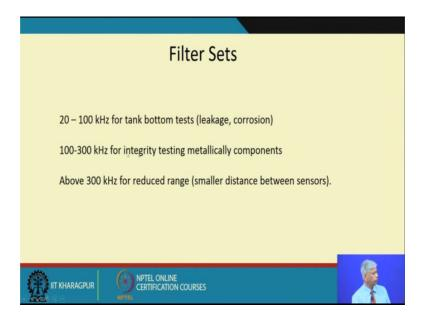
And of course, you can use a filter sets depending on your application because if digital signal processing is not available at high frequencies, we can use analogue filters ok.
