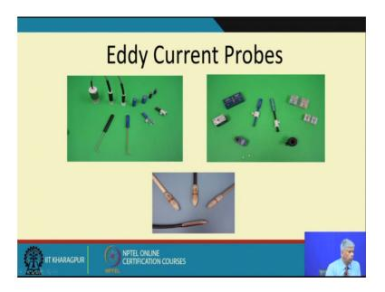
So, we can see the difference. So, typically this is how particular views of some commercially available Eddy current probes the common different forms and all you require is a Eddy current test equipment with multi frequency equipment and then you have an analogue meter and then recurrent probe.
