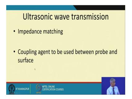
But most important is as a machine this impedance matching. So, coupling coupling agent is to be used between probe and surface and that is something one has to keep in mind.
