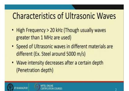
So, the characteristics of ultrasonic waves is there are high frequency typically usually waves greater than 1 megahertz are used. So, I can have ultrasonic generator which is nothing, but a piezoelectric crystal which is made to oscillate.
