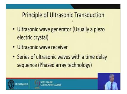
So, what how this ultrasonic transept transduction happening. so, this is nothing, but the wave generally usually a piezoelectric crystal and then we have a wave receiver.
