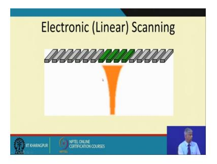
There is an example of the linear scanning, we are on charging them separately, I am not physically moving the transducer, but just exciting them the one by one the elements of
