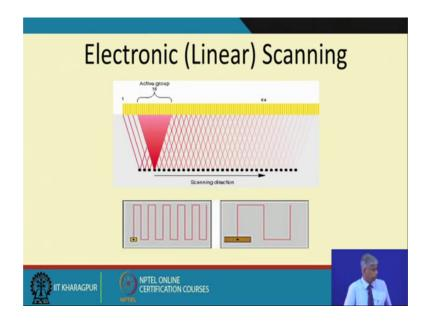
I can do linear scanning I can have the elements, but then electronically I can give a signal. So, that the elements do not move, but I will move this signal of excitation. So, I just place an electronic mosaic of elements on it do not move anything here, but move the excitation signal higher frequency and then do a scanning and so on ok.
