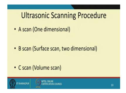
So, the scanning procedure there are names given for it A scan is a one dimensional scan, B scan is a two dimensional scan or a surface scan and C scan is a volume scan.
