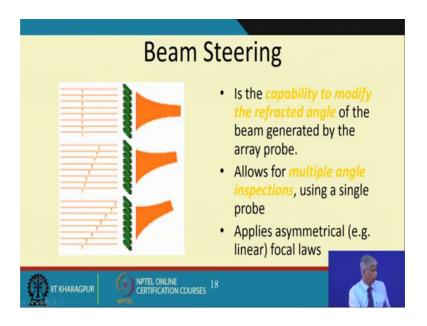
So, the beam steering can be applied as the capability to modify the refracted angle of the beam generated by the area probe allows for multiple angles inspection using a single probe ok. So, this becomes very easy for the user to do a scanning by ultrasonic.
