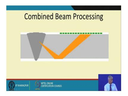
So, different phase there is scans are available ok. So, this is an weld effect. So, we can do that and so on ok. So, the entire depth of this weldment is scanned um, since I am moving it, this angle is not changing, but as opposed to this. So, we can scan the entire surface and this is what is essential when we do the weld defect scanning and. So, I can identify if there is a reflection here I can identify where this plot is. So, such arrangements are there ok.
