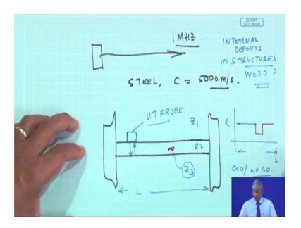
And generate a very very high frequency ultrasonic waves and speed is different in different materials, for example, in steel C is 5000 meters per second and the wave intensity of course, would decrease after a certain depth which is known as the penetration depth.
