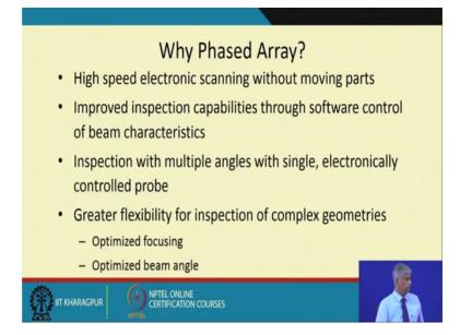
So, why phased array high speed electronic scanning without moving parts improved inspection capabilities through software control inspection with multiple angles with single and electronically control and greater flexibility ok.
