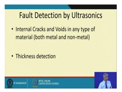
So, ultrasonic is used to find out internal cracks and voids in any type of material both metal and nonmetal though for nonmetal I will require a high power ultrasonic and usually for thickness reduction imagine on the outside.
