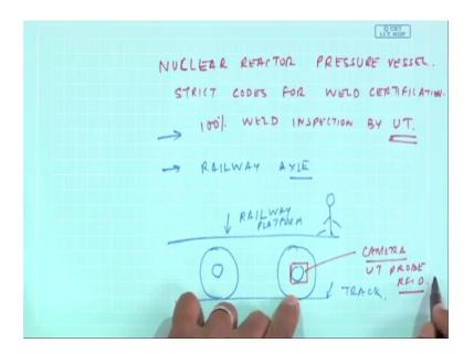
So in fact, some of the standards which are particularly used in nuclear reactors, nuclear reactor pressure vessel are very important components, they have strict codes for weld certification, they require 100 percent weld inspection by ultrasonics ok. I will just give you an example of the railway axial. So, if there was a defect in the axial, this could be scan and so on and today in fact, the idea is we can have such ultrasonic probes.
