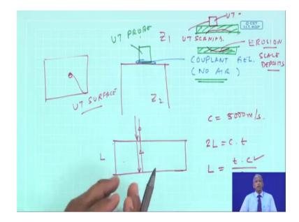
So, we put some sort of an gel because it this impedance Z 1 and this impedance Z 2 on this layer we put a couplant gel there is nothing, but a water based compounds. So, that there is no air between the interface of the probe and the material. So, to remove air a couplant and gel is applied and here also on this surface we are given a couplant gel. So, what happens how is it measuring the desert has taken as accurately is like this.
