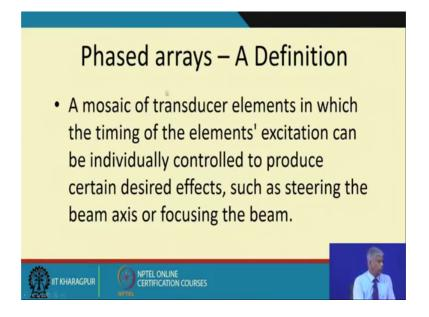
Phase; there is a mosaic of transducers elements in which the timing of the elements excitation can be individual controlled to produce certain desired effects such as steering the beam or focusing the beam, for example, I could be giving excitation I could timing it maybe I will illustrate it in the next diagram.
