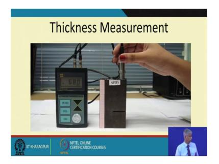
So, for example, here this is a steel block and we have artificially cut a slot here and I am putting this longitudinal probe by the way this ultrasound is very similar to the ultrasound you know people do or to find out baby in the mother's womb.
