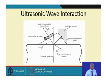
So, when I have a piezoelectric crystal. So, I will have an incident beam. So, job under inspection it will get refracted because of the density difference and then some will get reflected ok, I am not interested in this reflected beam rather I want to see how much of refraction is happening. So, I can put have an ultrasonic absorbing material here.
