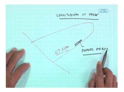
This fuselage ok; we can do UT scanning to find out or defect on the surface of the skin of the air long ok, of the flaps and then we can find out the faults by having such phased error technique.
