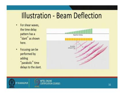
So, here in a shear wave the time delay has a slant pattern. So, focusing can be added you know I can steer the angle ok. So, all these are done through signal processing units and many commercial such handled and lasers are available ok.
