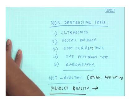
So, the non destructive tests which are prevalent in the industry for CBM, if I was to list them down Ultrasonics is one of them, then we have the acoustic emission, eddy current test, dye penetrant test, radiography. As you will see, these are not real time, but they have lot of engineering applications to find out the product quality bearing. Perhaps eddy current which could be used too as you have seen in the case of general bearing to find out the clearances ok.
