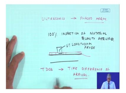
Now, recently a new technique has come in ultrasonics that is the phased array technology wherein rather than having a long conventional probe we have this something element cut into many many elements and each one of them could be energized to give an ultrasonic wave.
