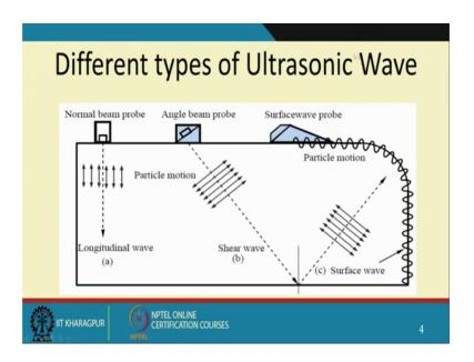
So, different types of ultrasonic waves and these are piezoelectric crystals wherein I can have a longitudinal wave here, did not I produce a shear wave. So, you will come across here and then get reflected because there is an impedance mismatch.
