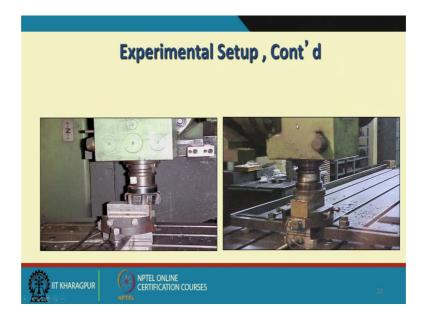
And this is another view of the cutting force dynamometer, put below the work piece and you can see this is the vibration transducer here.
