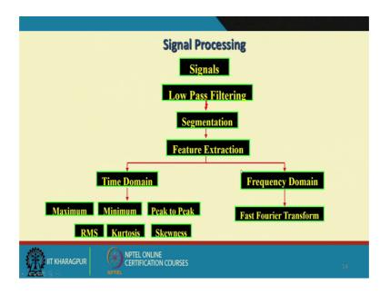
So, we did what is known as a little signal forcing a data driven. So, we did low pass filtering we remove certain artifacts from the signal, and did a time domain feature extraction these are the data analytics these are the features of the signal, if I have a signal coming from a transducer.
