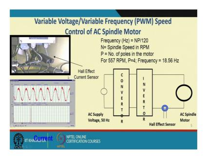
So, before I go into that I will also introduce you to our technique, wherein we measured this current through a Hall Effect sensor, this current is drawn by the spindle motor which is used for machining and as you see this is a sinusoidal signal, and there is a single frequency signal single frequency component.
