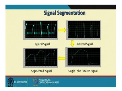
And this is what typical signal segmentation has done if you see here a typical signal there is a lot of information here and there is not much information here. So, and there is a lot of high frequency noise which was removed by filtering and will through a low pass filtering.
