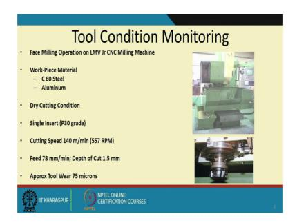
So, let me introduce you to what this is about. So, we have a machine or CNC milling machine single spindle, and then these are the conditions of the tool work piece one case there are steel and another case there was the aluminum, there was dry cutting this is single insert and we had cutting speed the spindle RPM set at 557 RPM approximate feed was about seventy eight millimeters per minute, depth of cut one point five mm and he tool wear was 75 microns to begin with ok.
