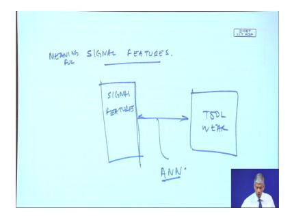
So, this request if I go back to the previous slide here, signals have been acquired from the transduces little low pass filtering to remove the noise segmenting, and then the feature extraction and use this parameters; these parameters of maximum minimum peak to peak RMS kurtosis Skewness these are nothing, but features of the signal or which relate the signal to the condition of that machine.
