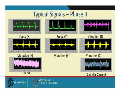
And this is the typical signal which is obtained from the sensors; force in x y z directions vibrations spindle current and so on.
