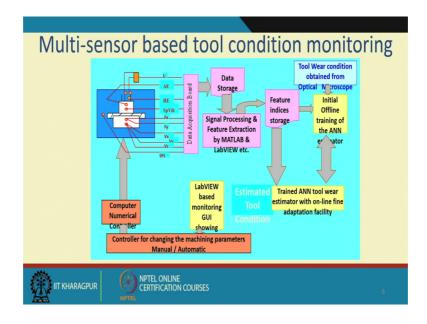
We did a multi sensor based tool condition monitoring, as to we in this machining operations we measured the acoustic emission, the high frequency, acoustic emission signals, the vibration levels, the forced levels, sound levels, the voltage current etcetera. So, everything was required I will not go to the details of how the acquisition was done something which we are going to discuss later on.
