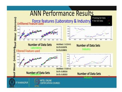
So, you see the tool wear in microns both in laboratory and in industry, we are able to predict better once we it has the filtered feature the instead of the unfiltered feature.
