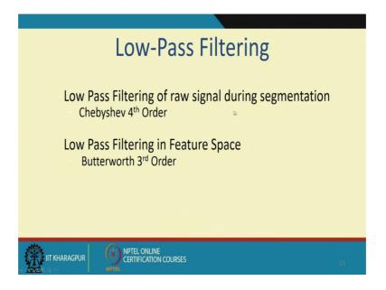
So, for the low pass filtering this was the filter order which was used.
