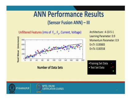
And then h with sensor fusion by sensor fusion I mean, it is just not force I took force current and voltage all of them together for having a robust model to predict the tool wear. And in fact with sensor fusion we have a better prediction. In fact, this paper is there referred to in my book.
