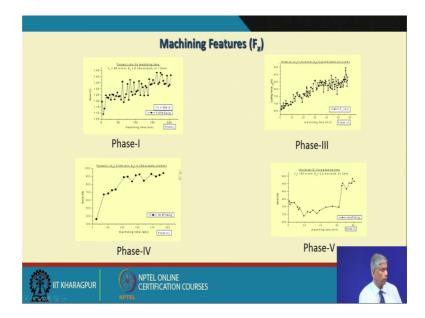
And then we looked into different in a 1, 3, 4, 5 these are the different failures of instance, where with machining time in the x axis we will see how the parameters like you know force the in different directions etcetera are changing as we will see, with the cutting tool machining time increasing the tool wear would increase.
