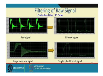
Filtering of the raw signal; so this is up to an individual how you want to do it, and this is what was used in our analysis.
