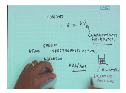
So, if we have a spectrophotometer which can measure the energy of these electromagnetic radiations at that characteristic frequency, I can know what kind of chemical element is there. So, such devices are known as spectrophotometer. So, one is an atomic emission another is absorption.
