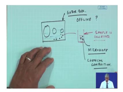
Suppose, I have a large gearbox, is a gearbox in outside and there is lubricant taking oil.
