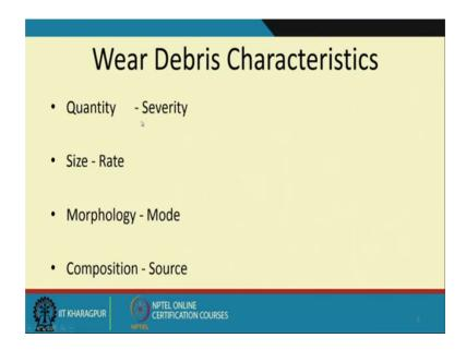
So, how do I know the quantity, there are devices by which you know we can see the particle count in terms of by a laser devices we can measure the particle count through an optical technique.
