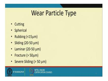
So, depending on the wear particle type there will be different sizes of this some the cuttings spherical or rubbing wear you know typically the sizes are very very less, may be 2 hour you know if you if you rub in your hand, the oil you will find that it is feeling rough of. So, this roughness is because of this wear particles are getting in the oil.
