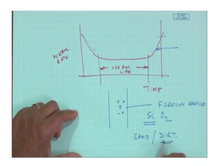
So, some of wearing modes you know you recall the bath tub occur with time wear rate and which we are defined this as the useful life period. So, the initial run in where we have an high wear rate and towards the last time the end of the life of the machine we have a high wear rate ok.
