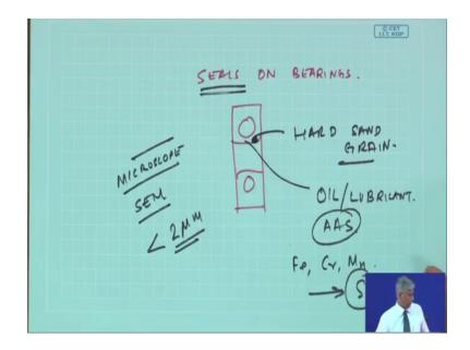
So, seals form on bearings because imagine, I have a bearing and one foreign particle gets trapped hard sand grain. So, this is going to score the races and it will form lot of pits. So, this has to be avoided.
