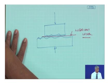
This is my lubricant layer. So, there could be addition there could be abrasive or cutting wear delamination fatigue after delamination occurs in composite materials fatigues corrosion or oxidation wear and electrical attack acid attack ok.
