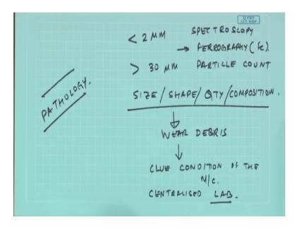
And more than 30 microns we can do just particle count sometimes inside is known as the ferrogram, but this is only good for ferritic or iron surfaces.
