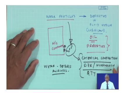
The fluid medium is lubricant. So, in the process, what happens the lubricant also get spoiled ok, lubricant are be can tell, it as oil. So, oil will also get contaminated. So, all something will the oil properties would change ok.
