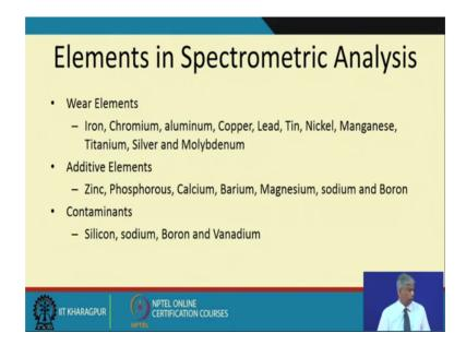
So, some of the elements in spectroscopy analysis we must know beforehand that these are the typical wear elements which we will find in any oil sample and some of this additive elements are used because of the composition and then the contaminants silicon is the most sodium and so on.
