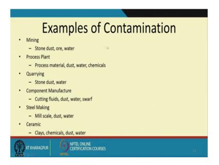
So, some of the examples of contamination are mining process plant query I was talking about you know querying stone dust water mill scale dust water. So, all these components will get deposited in the lubricating oil and then later on.
