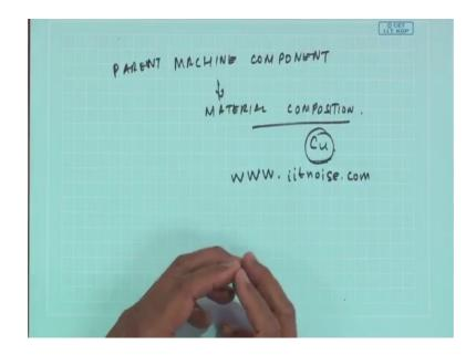
So, this will give us to a guide that if I see may be copper I know in a machine in a gearbox, I see copper will all be wondering you know in me in my first case perhaps there is no copper. So, where this copper come from maybe the general bearing in some bearing has copper because of the lining and then this copper came above.
