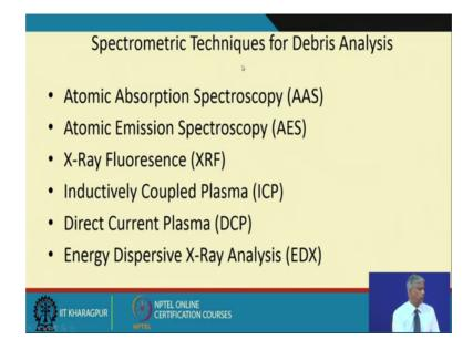
Some of the spectrometric technique used for debris analysis I just mentioned you atomic absorption spectroscopy or atomic emission spectroscopy XRF, SRD, ICP, DCP, EDX. So, these are some of the machines spectroscopic machines which are used for doing the analysis, but mind you they are very very costly couple of them could run to few crores or few less than crore.
