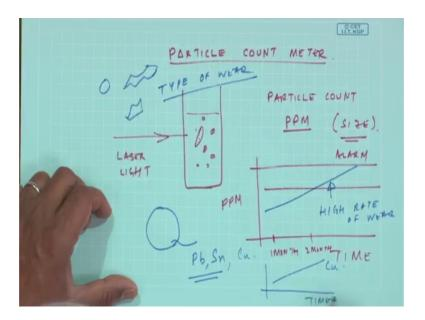
Suppose, I have a particle and then there are particles suspended in the fluid, if I shoot a laser beam and depending on the size of this particles in a given volume the energy will get reflected from this surfaces. So, I can have a clue as to the particle count in a given volume; so, parts per million of a particular size. So, such particle count meters are
