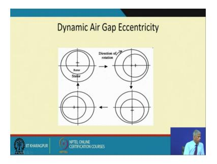
So, dynamic air gap eccentricity, you see, if it is rotating this gap is going to change, right so; obviously, the magnetic torque would change and then bent rotor shaft bearing has worn out misalignment mechanical resonance at critical speed.
