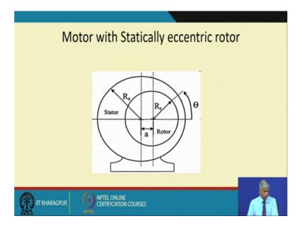
Now, similarly when we have motor with static eccentric rotor you see the centres of the stator and the rotor are not as the same point. So, there will be an ovality ok. So, this hobbling of the rotor in the stator and this creates an uneven gap.
