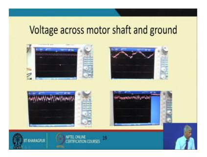
And I do not know if you can see these are very high frequency transients which could be removed and this is the normal motor very low voltage single frequency.
