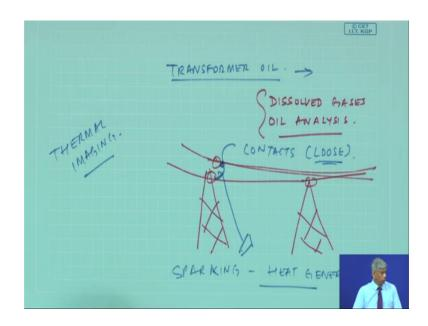
But if you look at this wire here the transformer oil is required to keep to transfer the heat because of the magno to resistive forces which is generated to be exchanged with the atmosphere these are the fins. So, what happens the oil quality would change with time? So, just oil quality has to be monitored we have a routine as to and of course, some dissolved gases which are there in the soil.
