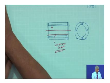
So, maybe, we have fault 4 bolt holes ok, suppose the end frames and both of them both these directions both the planes are not the same. So, there could be a eccentricity incorrect position of the rotor or the stator determine in current installation.
