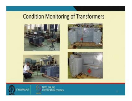
But then there are few other machines which I have told in the beginning in this transformer ok. So, in transformers what happens this is in a laboratory which I am trying to explain to you this transformer there is a we are measuring through laser based vibrations. Here if you can see here, this is a laser vibrometer and these are the spots wherein we are measuring the vibrations, but this is not humanly possible to always measure the vibrations.
