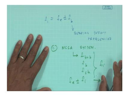
There will be some these are the bearing defect frequencies. So, just to monitor the defects in an electrical motor, if we have a MCSA system and if you know the rotational speed or the supply frequency, you can calculate the frequency because of broken bar
