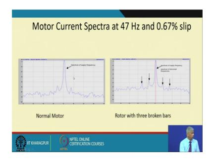
So, here in a motor being driven at 47 hertz with 0.67 percent slip, this is the normal motor and if you look at the current spectrum ok, though, there are few sidebands happening because the normal to begin with there could be some defect in the broken bar.
