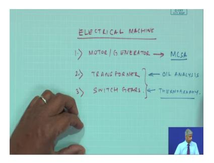
So, when I talk about electrical machine, I will broadly classify them as the motor generator, then we have the transformer and of course, the switch gears ok. So, we will focus primarily on motor current signature and passing, I will tell about transformer and switch gear actually transformer when you talk about oil analysis, we will discuss about them and this is very easily done by a technique called thermography which is nothing, but infrared imaging.
