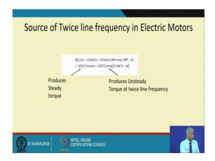
But another thing also we must see in the; in a line electrical motor, I had earlier told you that if the supply frequency is 50 hertz, I will see sometimes peaks at 100 hertz, this is because of the reason that if the supply frequency is a cosine function EMF is produces a phase difference. So, if I multiply them, the power will be have a cosine phi term and also this is a steady torque and produces an unsteady torque at twice line frequency.
