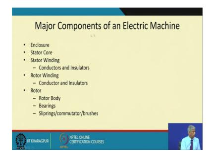
So, the major components of an electrical machine is the enclosure of the casing the stator core, the stator winding, it has conductors and insulators the rotor winding which has conductors and insulators the rotor itself the rotor body bearings slip rings commutators or brushes. So, that the current actually comes out of the motor or we supply them or and so on.
