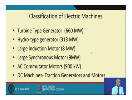
So, if you look at the electrical machines which are generator or motor, you know, they can be very very big; 660 megawatt hydro type generator, 313 megawatt large induction motor, 8 megawatt large synchronous motor, 9 megawatt AC commutator motor, DC motors and traction generators and motors and railroad locomotives etcetera, ok.
