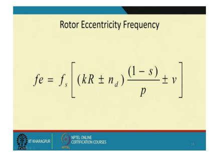
So, in such a case; the candidate for motor current signature analysis is this ok. So, these are again the same frequencies for the rotor eccentricity frequencies.
