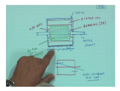
Now if you look at a motor, essentially, they have such a unit, this is the rotor which is supported on bearings and this is put in a casing where there is a stator coil and this is carrying a rotor coil and everything is there in casing.
