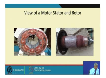
This is the view of the stator coils because there are pole pairs and then this is the casing and this is the armature ok, where there are the rotor bars and this is the bearing and this for generator this is the slip rings where we put the carbon brushes to take in the voltage output and these are all rigid.
