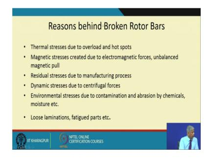
So, reasons behind broken rotor bars is thermal stresses due to overloads and hot spots magnetic stresses created due to electromagnetic forces unbalanced magnetic pull residual stresses due to the manufacturing process dynamic stresses, due to centrifugal forces environmental stresses, due to contamination and abrasion by chemicals moisture, etcetera, loose laminations fatigue parts.
