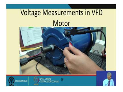
How does the VFD drive driving this motor just by grounding it, we could remove the transients which were occurring.
