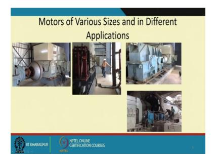
So, big blower there because as you know these motor bearings I had told you before should not be overheated. So, they need to be cooled and this is a person standing here. So, you can understand the height of the gear of the motor box and this is another motor which is driving a helical gear box bevel gear arrangement is there, this is a another motor which is driving the kiln of a cement plant.
