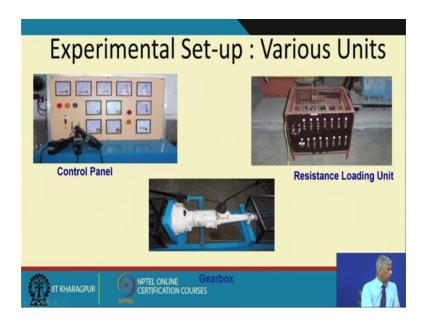
Then, automobile gearbox; where, I can induce defective gears. And then, see the current drawn by the electric motor.
