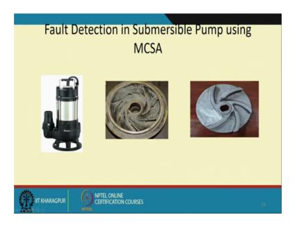
The similar thing which we did for the submersible pump also where we removed artificially the veins and then this was done at different impeller conditions.
