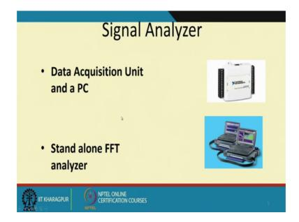
So, in terms of the signal analysis equipment, all I require is a data acquisition unit because is a very slow signal 500 hertz; I can I can capture with the data acquisition unit and I can have an standalone FFT analyzer or a laptop. So, comparatively this is a very cheap setup compared to the traditional vibration transducer. So, basically all you need to have is a computer with a data it can DAQ and Hall Effect sensor.
