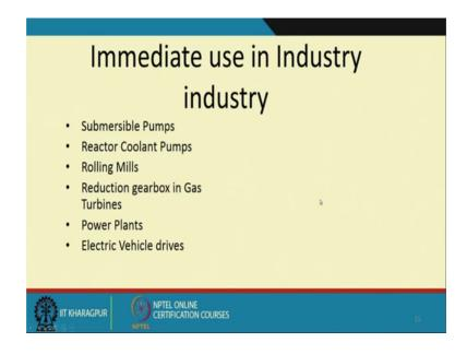
So, immediate used to the Indian industry is because, MCSA is remotely we can do we can use them in submersible pumps, reactor cooling pumps and in some nuclear reactor and rolling mills in large reduction gearboxes in gas turbines power plants and even today in electric drive vehicles.
