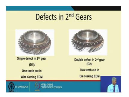
So, we have two cases D 0 no defect in the gear D 1 is one tooth removed and D 2 is two teeth removed. So, all these conditions we ran the gearbox at different speeds measured the current measured the virus and send then all the conclusions which we have got.
