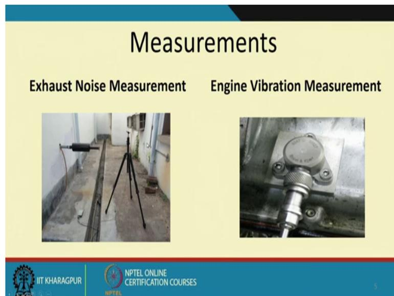
And at the exhaust side we have a muffler and then we have put a microphone here to measure the exhaust noise and in this particular example, we did not measure the cylinder pressure rather measured the engine vibration by a high temperature accelerometer, by the way this accelerometer is very costly and you can measure all the way up to 600 degree Celsius using such an accelerometer and you can see because of high temperature all this cablings arrow all metallic sealed in metals.
