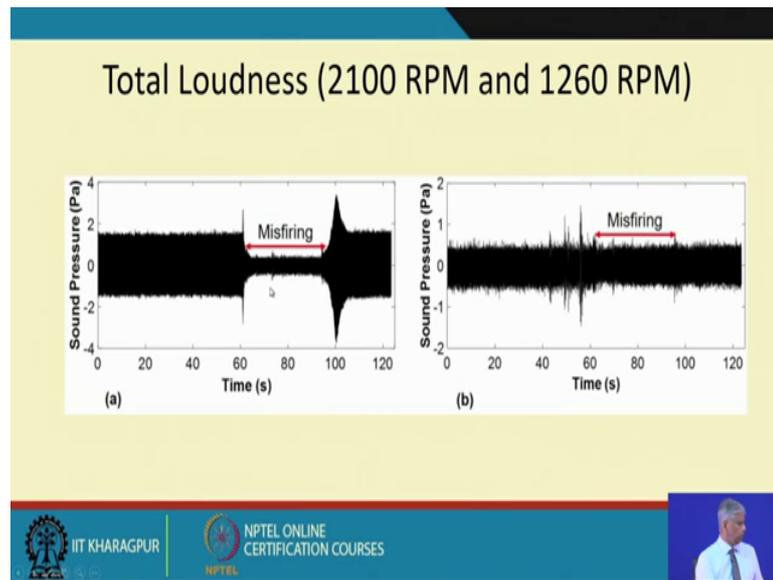
So, you can see right away there is a typo here, the should be a sound pressure here sound pressure here. So, you see the sound pressure here there will be the case of misfiring at a low RPM, there is a misfiring, but the sound, we are not able to detect visually in the time history both the amplitudes are low as compared to the sound pressure which drastically reduces at high RPM because of misfiring and at the end of about thirty seconds we again switched on the engine.
