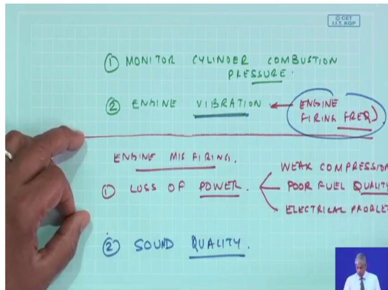
And so, from the to measure the cylinder pressure we actually have the pressure sensors which has to be put inside the cylinder which can withstand the high pressures and high temperatures which occur inside the combustion chamber or alternately we can measure the engine vibration ok.
