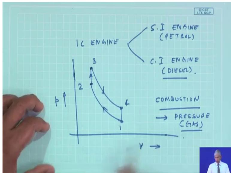
If you classify IC engines, there are through broad classification the SI engines in the petrol spark ignition engine and the CI engine and the diesel engine the compression ignition engines ok.
