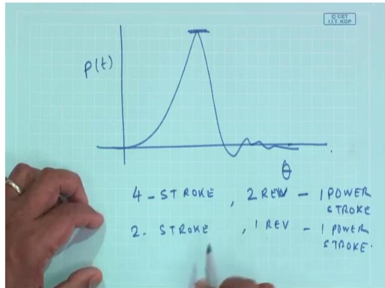
And this is the prime mover this combustion of the fuel is responsible for giving rise to a pressure and it is this pressure which is responsible for the power and so on and then of course, in 4 stroke engine, we have for every 2 revolutions 1 power stroke and for a 2 stroke engine, we have for every revolution on power stroke.
