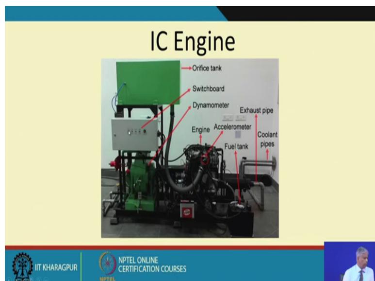
So, this is are typical engine where you will see in our laboratory this is a 4 cylinder engine which is coupled to a dynamometer and there are 4 cylinders there are 4 switches here which can switch off the electrical supply to the spark plug of this engine. So, that I can create a fault by what is known as engine misfiring and of course, you will see there is an water cooled engine.
