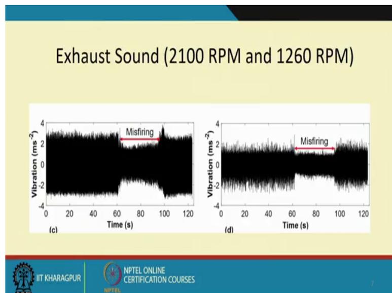
So, I will give you an example in this case here of course, in this laboratory as a case study we ran the engine at many different RPMs and I have just given you two representative rpms one being at twenty one hundred RPM another being at twelve sixty RPM and the vibration was collected by that accelerometer measured by the accelerometer for about two minutes and I must tell you that this is a normal engine and we artificially misfired one cylinder.
