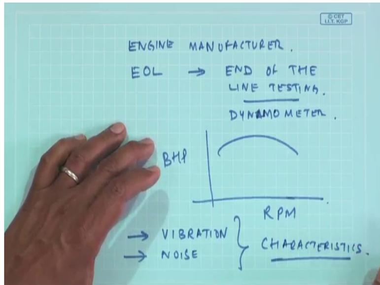
They do what is known as EOL and of the line testing maybe on a dynamometer to see the RPM which is the BHP curve, whether it is producing as for the design specs, but sometimes even monitoring the vibration or the noise and looking at the characteristics you can find out the faults in the system.
