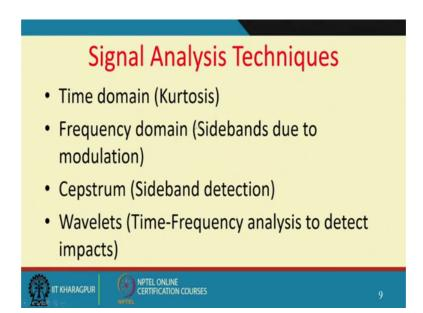
So, some of the signal analysis techniques which are used, I can still do kurtosis because there is a lot of pickiness in the signals frequency domain analysis side bands due to modulations and modulation occur because of amplitude effects.
