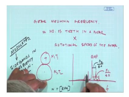
GMF stands for gear meshing frequency and which is nothing, but number of teeth in a gear times rotational speed of the gear. Now, what happens if the gears are meshing, this is N 1, T 1, N 2, T 2, if I and because of load these signals are modulated and as you recall modulated signals in the time domain will give side bands in frequency domain.
