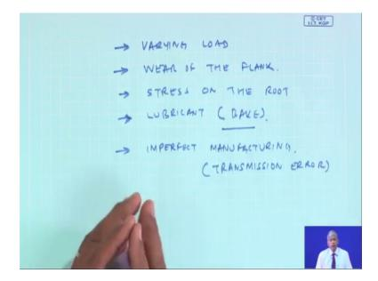
So, a gear under load will be subjected to varying load will be subjected to wear of the tooth flank wear of the flank of the gear stresses on the route will develop and then will of course, in the lubricant can again bake like the example of gear like the example of bearings which you discuss about.
