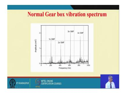
So, this is even in a normal gearbox out of the rig in the laboratory which we saw, we can see such gear meshing frequencies coming up.
