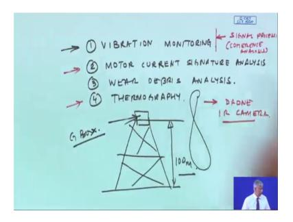
Now one is vibration monitoring which you will focus this class on and another technique which has emerged lot of the research at IIT, Kharagpur is using motor current
