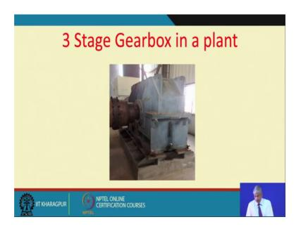
This is another 3 stage gearbox in a plant there is some view which I am going to give you, you can see there is a motor here and motor is along into the plane of this projection here, but do you see there is a 90 degree turn in the power direction. So, we have a strong
