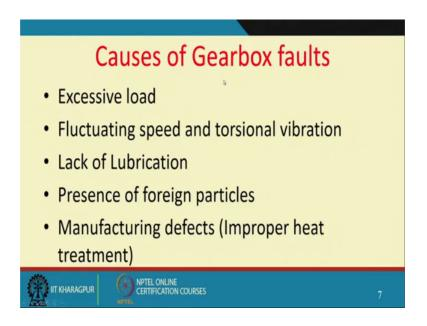
So, what are the causes of gearbox faults excessive load fluctuating speed and torsional vibration, why does fluctuating speed occur by now, you must have got an idea why fluctuating speed occurs one is the prime mover.
