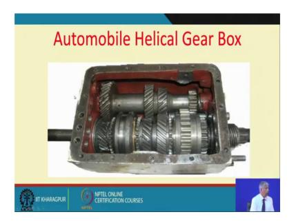
So, the one is an input shaft with a gear and another is the lay shaft depending the gear you shift and this gear should shift and then the corresponding speed ratios would be selected. So, he could be having a gear shifter which will change the machine gears. So, and then you can have a first gear second gear third gear fourth year and so on or a reversing gear and then of course, you know this is the spur gear and this is a helical gear and so on.
