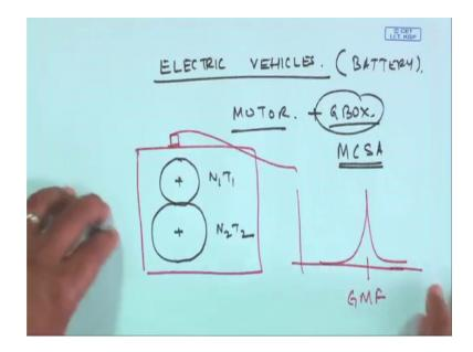
So, how do you monitor the gearbox of such electric vehicle and MCSA is a good area by which MCA motor evolution can be done.
