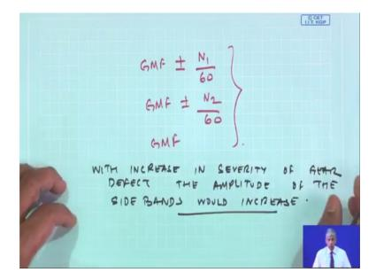
So, what happens the amplitudes with the increase in the severity of the defect, let me write this down with increase in severity of gear defect the amplitude of the side bands would increase.
