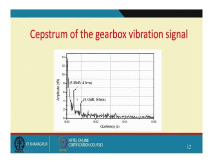
So and to detect the particular gear all you require is the septum analysis given in quefrency and if you see 4.8 milliseconds or 9.6 milliseconds and there is an amplitude. So, this means the gear which is having a time period of 4.8 milliseconds is severely getting affected. So, if I monitor this amplitude over a period of time in a gearbox where
