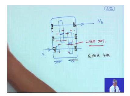
So, if I have a gearbox and as you know, suppose this is a gearbox this is my input shaft there could be an intermediate shaft and there could be an output shaft and so on, this could be happen ok.
