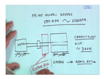
So, the prime mover speeds typically from 500 RPM maybe to 6000 RPM this is what happens, but the mechanical unit which are being moved by this prime mover may have a requirement of another speed like in the case of a cement plant the kiln maybe rotates only a 3 RPM ok, in automobiles, we require different speed ratios speeds.
