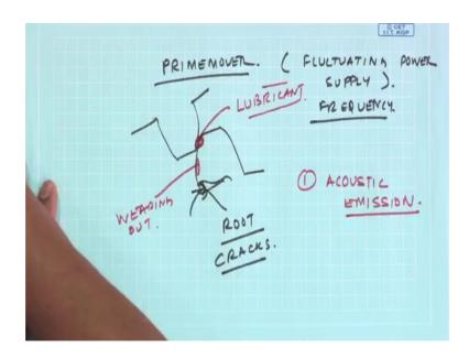
It could be fluctuating power supply in terms of the frequency if there the case of an electric motor. So, this will all give rise to torsional vibrations and then there will be excessive vibrations lack of lubricant because if you see the gears which are meeting there is always contact.
