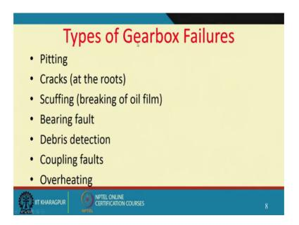
So, these are how gearbox faults occur. So, types of gearbox failures pitting cracks at the root scuffing is what is known as braking of the oil filling a bearing fault the bridge detections coupling faults and overrating. So, these are all are responsible for the bearing faults.
