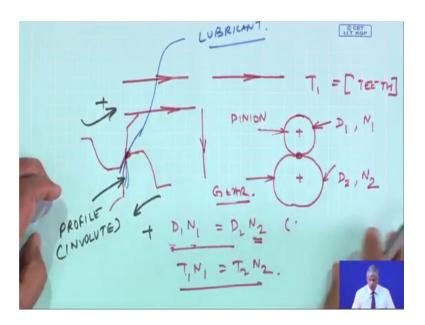
So, gearbox forms a vital component in any mechanical plant or industry and another complicated problem is the power direction. Sometimes, the power is in line, sometimes, I need to have the power direction changed. So, this forms that the speed reduction will be there and as you know from the law of gearing, if I have pinion meshing with the gear, the pinion has a diameter D 1 and its speed is N 1 this has a speed D 2 and speed N 2 speed N 2 means rotational speed.
