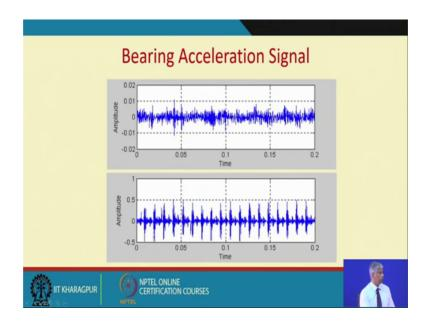
So, this is the typical example of the vibrations coming out of a good bearing acceleration signal, you can see the amplitudes are low the pretty much periodic, but this is for a bad bearing vibrations you see the amplitudes are high and they are periodic in nature is impacts hitting every rotation the impulse are been generate because some rolling element or ball is going and coming and hitting against a defect in the races or in the ball.
