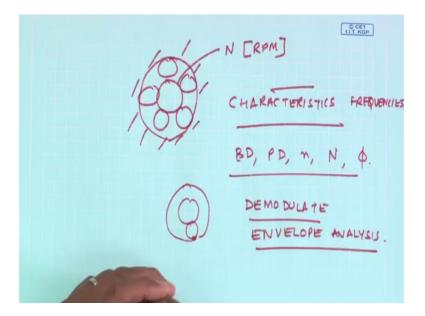
So, on top of it, if you look at the bearing dynamics, if this shaft is rotating at speed N RPM and if they are all held all these individual components will rotate at their respective characteristic frequencies. So, if you look at the bearing vibrations both new bearing and good bearing, you will see the statistics frequencies and then the bearing vibration itself is a complicated and so on and then I will show you some of these examples.
