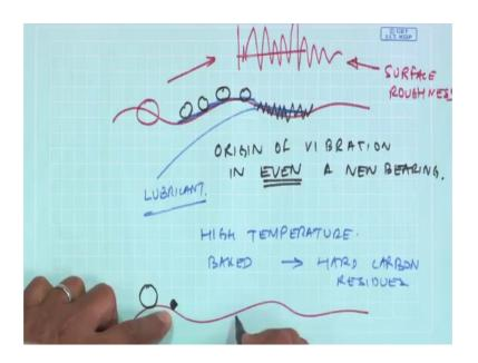
So, imagine I am having a rolling element and then you rather have a series of rolling elements which are moving on waives surface with surface roughness. So, this is the origin of vibration in even new bearing on top of it. So, to reduce this vibration what people do are there in manufacturing they put a layer of lubricant to remove the surface of spirit is. So, lubricant is put and the bearing are sealed for life ok.
