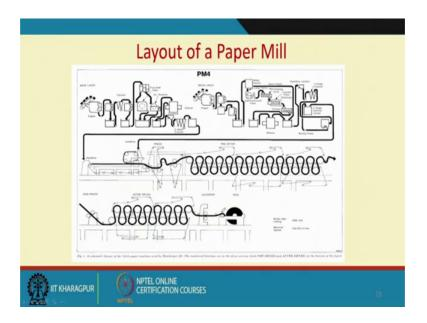
And then I will discuss about this paper mill, etcetera, in the subsequent class when we do vibration monitoring of are the case study in paper mills and how important it is. So, you can as you can see there are so many rolls supported on bearings and imagine if one bearing of a roll filled the plant had to be shut down. So, we will discuss this in the case
