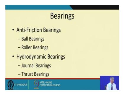
So, this antifriction bearings are can be either ball bearings or roller bearings or tapered roller bearings and these bearings always have direct contact for the surfaces which are in contact has to be hard and has to be polished to finish. So, that the friction is the least.
