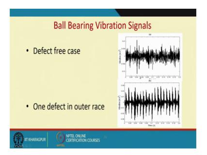
So, this is the defect free vibrations. So, people can develop I for your not even looking the frequency spectrum just looking at the time domain of the signals just looking at the ball bearing vibration signals and then the outer race defect frequencies.
