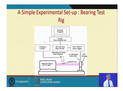
So, we just discuss about these and those of who want to do certain experiments in the laboratory, this is actually bearing test rig, we have a motor driving the housing where there is a bearing we put in accelerate meter to the power supply we have a filter and then we have data acquisition system and then personal computer we have an photo electric probe to measure the steep.
