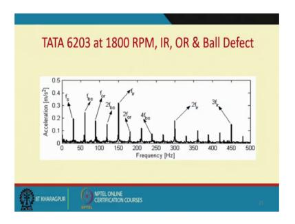
So, in see if you can clearly identify, these defects frequencies from the measured vibrations signal and if you see high harmonics it is the one way of knowing that the defects has occurred another is definitely mountain the high frequency vibrations.
