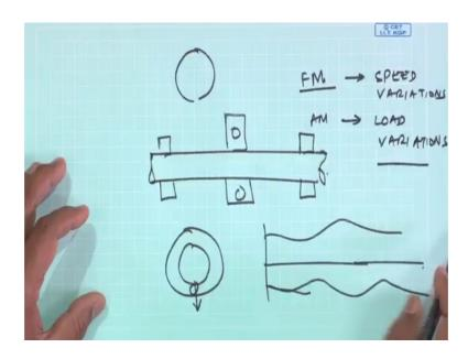
The bearings are supporting there is an unbalanced load.
