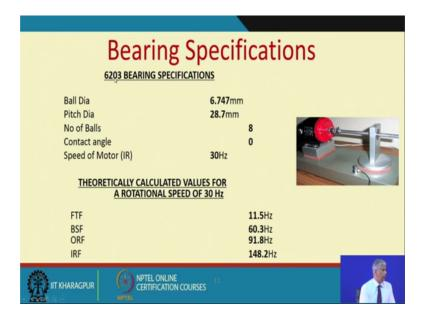
So, for a typical 6203 bearings which was mounted here some of the dimensions are here using this equation, the fundamental train frequency, the ball spin frequency outer race frequency inner race frequency for a speed of 30 hertz, these characteristic frequencies are calculated and if you see this spectrum of the vibration.
