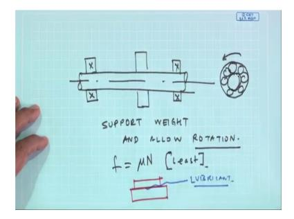
I have a shaft and then shaft could be a member of a machine component which could be carrying a gear or pulley, etcetera, but the shaft to be supported on a bearing which I am indicated by this process.
