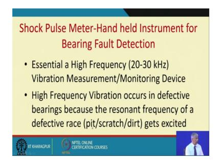
But, essentially the high frequency vibration measurement. Because high frequency occurs because of the resonant frequency which gets excited because of the defective race like a pit scratch or a dirt.
