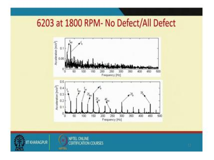
These frequencies will show up in the vibrations spectrum measured at eighteen hundred RPM correspond to 30 hertz. This was measured in a laboratory, this is the case when there is no defect and then you can see only the rotational speed of the inertia speed
