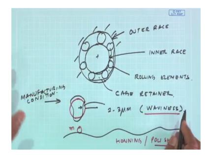
So, the major components of a rolling element bearing are like they are manufactured, this is the outer race, this is the inner race and in between the outer and inner race, there are rolling elements which could be balls rollers for tapered roller rolling elements and then there could be retainer or cage. So, that is ensure that no two rolling elements come in contact with each other and they are actually stand metal cage or retainer.
