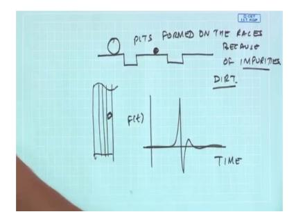
So, I can have pits formed on the races because of impurities one shot of impurities is this carbon residue another form of impurities could be dust or dirt ok.
