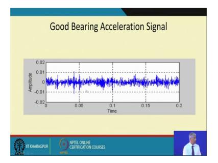
So this is the good bearing vibration signal amplitudes are low by the way they are deterministic periodic signal because of the variations and then with the outer race defect
