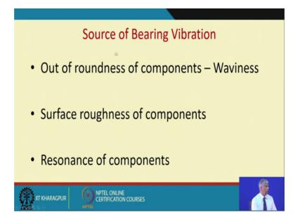
Now, so, we know the sources of bearing vibrations is out of roundness of the manufacture components or surface roughness of the manufacture components and then the resonance of the components.
