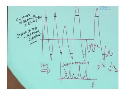
It will be so high 1 reason is the data efficient system has a limit to how much it can take. So, these are responsible for clipped vibration signals or what are known as truncated vibration signals. So, these kind of truncations will give rise to what is known as clipped
