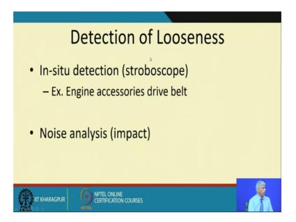
And while we talked about stroboscopes I had given in examples how detection of looseness can be done, using stroboscope if when engine accessories belt is slipping etc and noise analysis can be used to find out defects.
