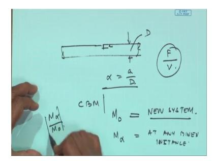
This is the shaft diameter d sum a, s alpha is nothing, but a by d for such crack depth ratio this has been normalized, we measured the change in the mobility and this was published in 2002 here almost more than 1 and half decades. Now also very popular
