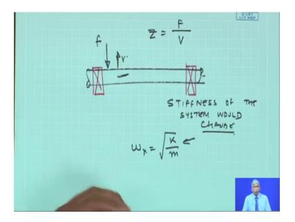
If system changes what happens in as you know omega n is root of k by m. So, if the system stiffness changes the natural frequency would change and that would mean the Eigen from an Eigen value analysis. We can do that another is if a systems property has changed I can measure it is impedance, what is this impedance is nothing but force by velocity. So, for a system I can give or known force f I can measure the response v;
