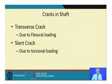
So, the shafts can be transverse or can be slant or and so we will see.
