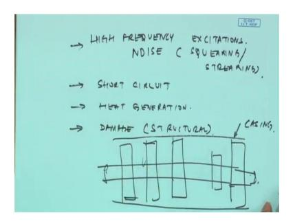
So, happen because of such rubs eventually this coil can get shorten, coil there will be heat generation short circuit, heat generation because of rub and eventually damage structural damage imagine. You know you are talking about large turbine with many sets of blades and range, so lack of space I have not drawn all of them in the direction, imagine if this touches the casing because there is a radial plane.
