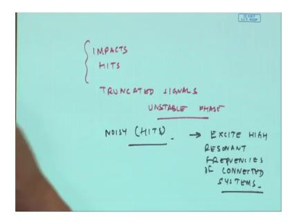
So, lot of impacts hits will occur give rise to truncated signals and unstable phase and from a noise analysis you will see lot of noisy hits and sometimes what happens because of this they will excite high resonant frequencies of connected systems, sothat can occur also occur.
