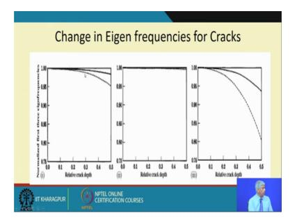
So, these kind of signature will lead to the changing in the Eigen frequencies of the crack because, I was telling you the natural frequency would change because of this factor k by m, so for the present Ks alpha.
