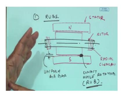
See rubs so happens for example if I have a shaft, particularly this has lot of effects. So, for example, if I have rotor of a motor inside stator, this is the rotor this is the stator of a motor. So, basically 1 is creates a magnetic field and this air gaps are very there to be uniform air gap that does, the magnetic reluctant and then the rotor moves to the magnetic field and that is a different story, but imagine if this bearings which are holding
