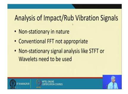
So, analysis of impact rub vibrations signals are non stationary in nature convectional FFT is not appropriate non stationary signal analysis like STFT or wavelets need to be used.
