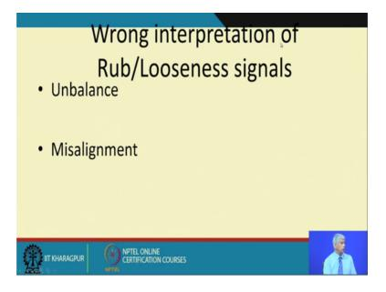
So, sometimes wrong interpretation of rub and looseness signals keep will you know call them as unbalance misalignment, because we know everybody does not have access to non stationary signal analysis tools. So, grid signal processing or beat analyzer, so this can happen in industry. Never the less they are non stationary and we have to use certain
