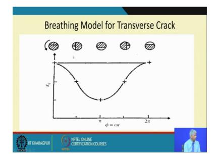
And then for a transverse crack some of the breathing modes are there it is change with the rotation of the shaft and this cracks will open and close depending on what position they are.
