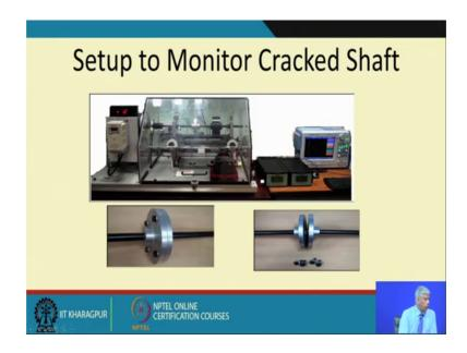
So, in the laboratory again same machinery faults simulator, we are in if you will see here we have a shaft and this black desk is actually a desk which is used to load the shaft and this shaft is actually simulated with cracks there are this 2 plunges you know aluminum plunges and if you see there are this 4 bolts and if I remove all the 4 bolts the 2 shafts will come apart and if I join them the 2 shaft will be a forming to a single shaft.
