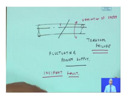
Because of the torsional variations particularly in many of the torsional failure, many of the rotating systems because fluctuating power supply leads to the variation of the speed, on top of it if there is a crack this will lead to an immediate failure of the system.
