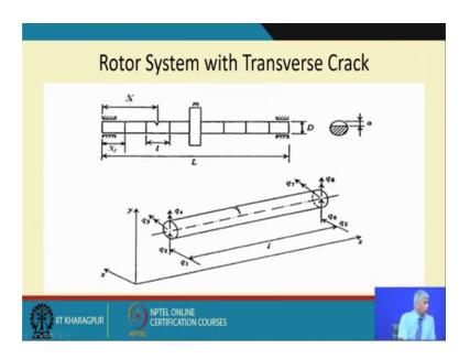
So, this rotor system with transverse crack was modeled by fire and elemental methods and this is that normalized I mean distance a. So, alpha is a by d or a by prime a bar is a by d and so on. So, this could be modeled in the techniques of fire and element method.
