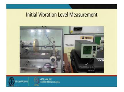
The same kit this is machinery fault simulator which we can have by the way this machinery fault, simulator is almost very popular in every universities and so on; where in we can simulate many experiments and many of the results which am going to share with you in this lecture series or in this course are out of experiments done on this rig..
