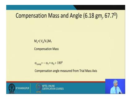
So, if you denote as a travel axis they should have been not there ok, it could have taken from the reference axis we can do it either way and then balance it. So, this is one way of balancing a shaft, just by having one measurement without stopping the machine and you know at once and put a trial mass and measure 2 responses and then measure the phase
