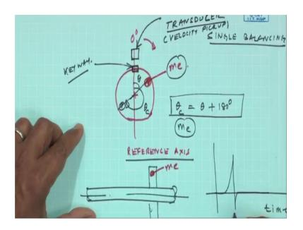
How do I create or unbalance, suppose there is an unbalance mass me, so with some reference suppose this is my 0 degree with some reference axis, I need to know what this angle theta is and then what is done unbalance amount.
