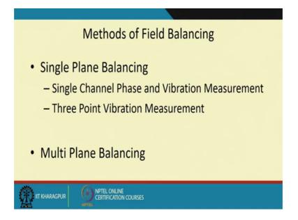
So, there are what we do we have to do in that case what is known as do a field balancing. So, without removing the disc from rotor we will balance it and there are balancing can be done in either in single plane or multi plane, if it is a long rotor this could be doing in balancing could be done in multiple planes or we can do it in single
