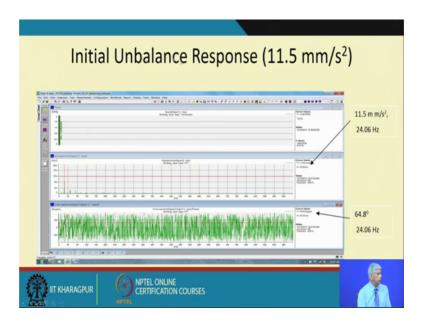
Then we measure the initial un balance response by taking the transfer function.
