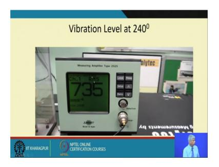
And we measure the vibrations at 240 degrees at 7 and 35 millimeters per second square.
