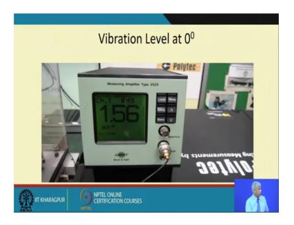
So, continuing with this we measure the vibration at 0 degrees we get a value 1.56 meter millimeters per second square.
