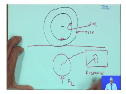
Am not drawing the well let me draw the tire excuse my drawing it is not a perfect circle is a. So, imagine if this was an every bit of unbalance in the tire and the vehicle was going on a road. So, every time the vehicle is going to get subjected to a force and this force going to transmit and then it will excite the response in the body ok. So, this response may not be desirable, so in people in NVH that is noise vibration and harshness.
