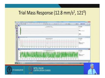
Will measure the trial mass response as 12.8 millimeters per second square and 121 degrees and then we will calculate the compensation mass as V naught by V T times M T and the compensation mass measured from the trial mass axis is given by from the trial masses ok.
