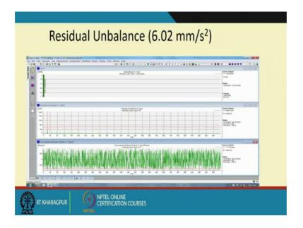
The residual unbalance then came down to about 6.02 millimeter per second square and it all depends on how good your travel mass is how sensitive you are to the initial mass and so on and this one of the very popular ways of balancing single plane balancing in systems. And the another method of balancing is known as the 3 point balancing.
