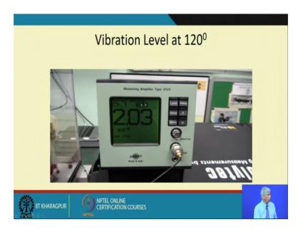
We measure the vibration level at 120 degree as 2.03 millimeters per second square.
