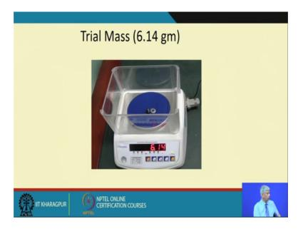
Then we will put a trial mass of 6.14 grams to the system the trial mass has been attached.
