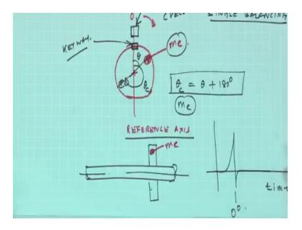
So, this signal must be 0 degree and then from there I can. So, always whenever I have theta correction I will measure my theta plus 180 degree from this point. So, this is very important and at the first step.
