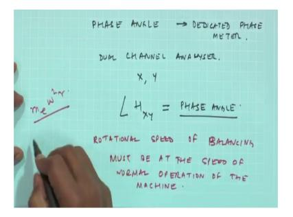
So, if I have 2 signals x and y, I can find out the angle between h x y and that is the phase angle and in the last class I had told you how we can calculate that and for us the dual channel FFT analyzer calculates phase. So, the first point is mark the location below the rotational speed measurements on the shaft as a reference point as 0 degree. So, this
