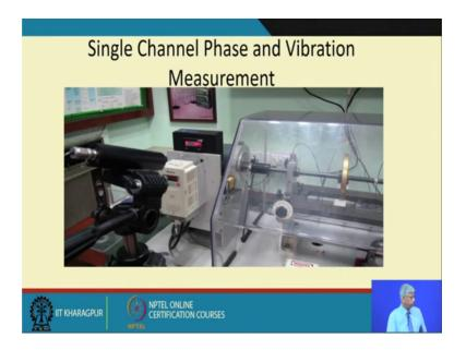
So, this is how this signal channel phase and vibration measurement is done in the laboratory. So, I will have a rotating shaft which at disc, wherein I can put in a known unbalance mass just for the sake of discussions here and this is the accelerometer which is kept on the bearing housing, this is a tachometer a tacho probe to measure the reference axis on the rotational speed.
