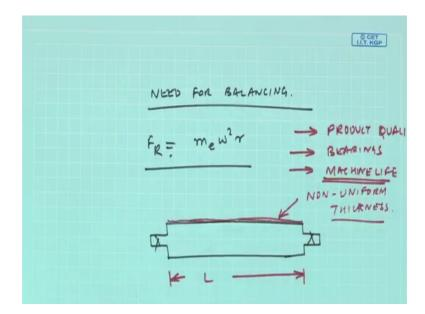
Balancing because, it gives rise to an radial unbalance force and which could load the bearings which could create un uniform deformation in rolls. This a role and if there is an unbalance if it is a long roll some length like in the case of a paper mill, the number of rolls if there is an unbalance the thin layer of paper which is there can have an non uniform thickness..
