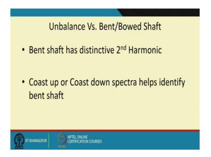
As opposed to shaft being unbalanced there could be a scenario where the shaft is bent.
