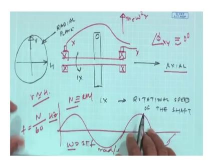
So, if I was to take a shaft supported on bearings, I will because of; so, you see this is my axial direction and this is the radial plane where I have the horizontal and then this is the vertical.
