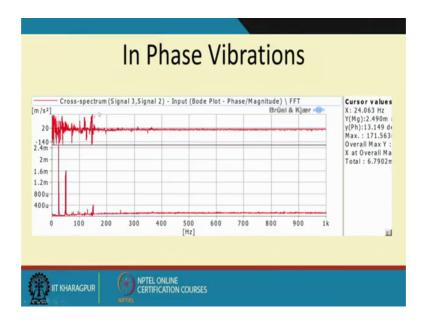
Now, this is just to give you an example where we have measured the cross spectrum between 2 signals and you will see the phase angle is only 13.149 degree this is subject to other unbalances in the system.
