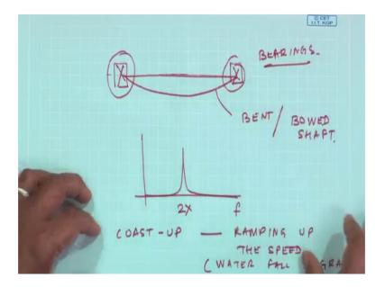
This my original shaft, but it has bent or bowed these are the bearings bent or bowed shaft.
