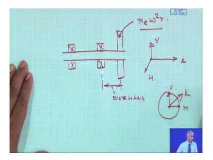
But when there is an overhang rotor supported on bearings and have a disk put here which is at an overhang and there is an unbalance mass there could be a strong axial along with the radial. So, in the real radial plane I will write H and a V and then axial vibrations may be on steady because it may not be uniform and axial phase may be
