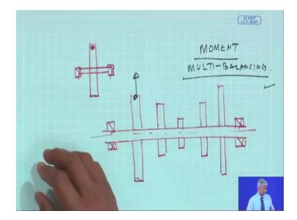
And I have just significant force in the radial plane, this a good example of static unbalance. So, it is unbalance in one plane as opposed to think of a large turbine in a power plant, I have a long shaft where there are stacks of blades and heavy, these are all stacks of blade later on I will show you photographs of you know gas turbine were you will see how closely this blades are there and.
