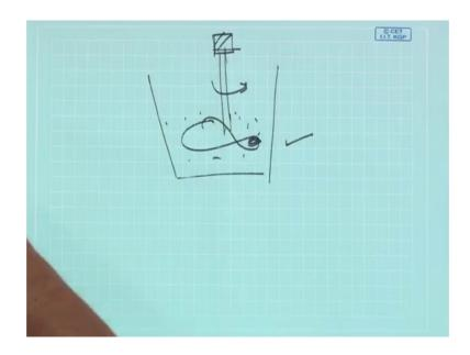
And we have large fan which is rotating supported lung bearings and there is some liquid here what happens something get stuck here the loads will come and there will be wobbling, etcetera. So, one will lead to the another such kind of faults occur and if I was to classify this one in to the static unbalance, another is known as dynamic unbalance for example, if the shaft is very small.
