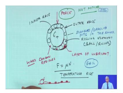
Now, imagine a bearing, those a few had a course in machine design will know a bearing have see this is my outer race this is my inner race and this is my rolling element which could be a ball or a roller what happens because this are all very hard nice surfaces we have lot of lubricant a layer of course, there is a returner which I have not drawn layer of lubricant.
