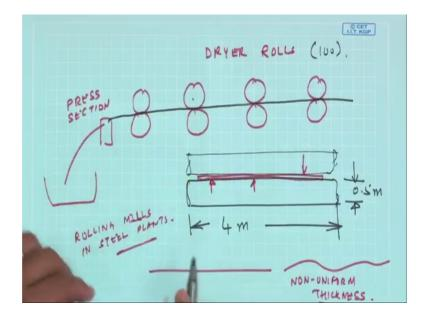
There are many rolls, this could be hundred such rolls and this is a there are process is there press a press section and these are nothing, but the dryer rolls which are steam heated in the inside and the paper which am drawing a black line here go out. Now, if you think of each of this rolls this rolls are the order of this is about four meter long and this diameter could be about you know of a meter imagine this paper which am denoting as here.
