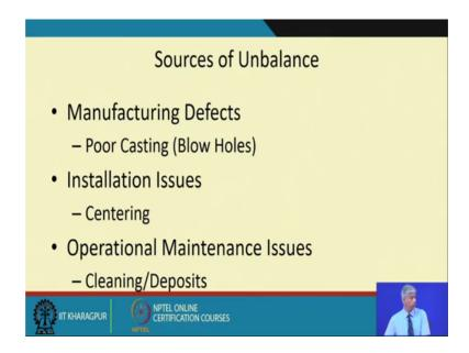
Now, question is in a first place why did this unbalance occur it could be poor casting imagine a pulley which is mounted on a shaft if there are blow holes because pulleys are usually cast.
