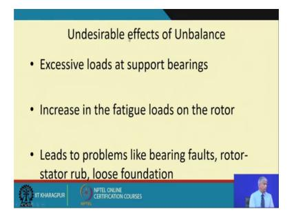
So, undesirable effects of unbalance excessive loads at support bearings increase in the fatigue loads on the rotor as I just told you leads to problem like bearing faults rotor stator rub loose foundations. So, these are issues scenario because know foundations will become loose because periodically there is a force which is hitting on the bearings ok.
