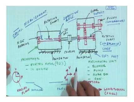
Now, if you will realize, essentially any rotating machine is actually combination of a prime mover which is mounted on a foundation and prime mover could be a motor or an engine which is coupled on to a mechanical driven unit which is again put on a foundation. Now each of this machines would have rotating shaft which I am drawing by
