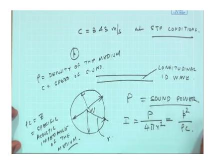
Now, for air this speed is 343 meters per second at STP conditions, they should vary with the temperature and so on.
