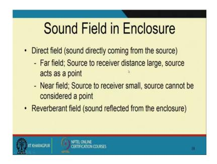
So, sound field in enclosure there is a direct field sound directly coming from the source, far field is source acts like a point near force source cannot be considered as a point.
