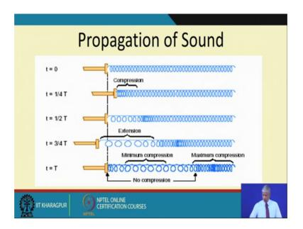
Now this is what I meant by the propagation of sound as longitudinal wave, so there are compressions and with time there are extensions are which are known as rarefactions. So, the entire time period of the signal or of the wave is nothing but if I show it as a transverse wave with time.
