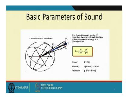
But then if you there is sound particle P and where I had told sound pressure P, where I have told that the pressure is only moving in one direction predominantly and that is a longitudinal one dimensional wave. I supposed to imagine if I have a point source P of some power this energy is going to radiate in all directions around the sphere.
