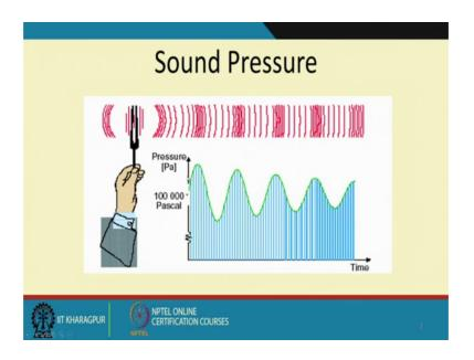
So, if you think of this sound pressure it is nothing but a small of fluctuation pressure in the ambient fluid, which travels from a source to a ear at a particular wave type.
