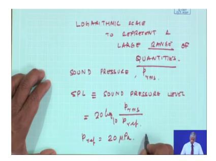
So, for sound pressure P which is p rms the levels are actually represented by what is known as SPL sound pressure level is given as 20 logarithm to the base 10 of P rms by P reference, where the international standard is P reference is 20 micro Pascal's ok.
