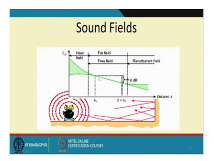
So, sound fields in the free field is actually we have the condition where the sound processer level decrease by 6 decibels and all the measurements sort of machines have to be actually done in the free field and if you go close to the boundaries they will reverberate or they will reflect and the sound levels may increase.
