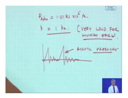
So, if P atmosphere is 1.0133 into 10 to the power 5 Pascal's, on top of it small pressure given 1 Pascal is very loud for human ears, so that is what we have to see. So, if you will see here this is the small fluctuation in pressure which is being incident.
