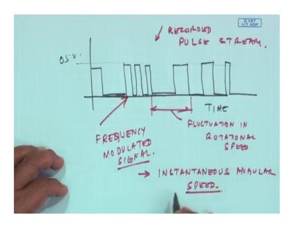
So, imagine if this pulse train and if I look at a very magnified view here it may. So, happen even in one duration the spacing would change the amplitudes are same. So, this becomes in other words frequency modulated signal and by analyzing this with an method called the Hilbert transform, which we have studied earlier. I can find out what is known as instantaneous angular speed of the shaft. Excuse me now, the question is why this time change?
