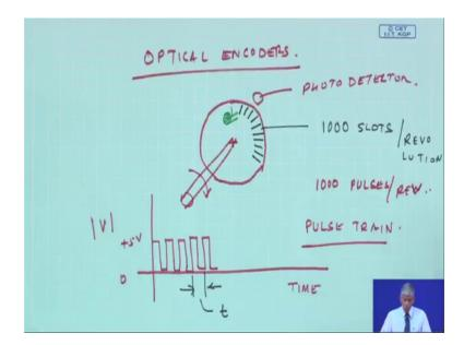
See, you see you are getting a feeling that without even monitoring vibrations just by carefully measuring the rotational speed of systems which are moving at a constant speed. If there is a fluctuation in speed, we can get some clue as to with condition of this machine. Right and if I talk about optical encoders see optical encoders are nothing but a disk which have slots on the perform on the periphery I am not drawing all these slots, but all around they are.
