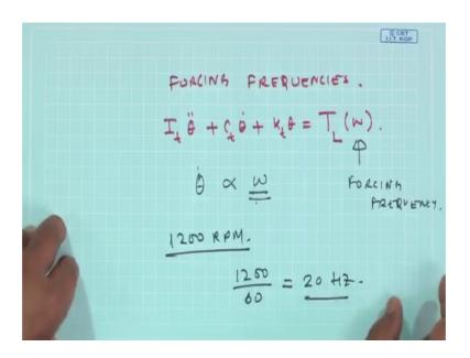
As you know, for any system you know if I if I write it in the rotational domain sum it theta dot plus Ct theta dot plus k t theta is equal to sum load torque TL which is a function of omega; obviously, this theta etcetera will respond at omega.
