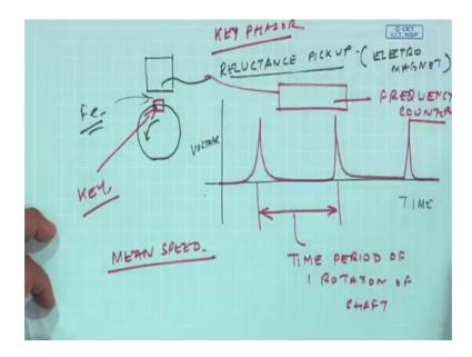
See, every shaft they have a key way if I put a key here and I put a pickup or reluctance type electromagnetic pickup. Of course, there is a casing in all that so, this is a reluctance pick up. What happens with the shaft is rotating? Each time the key comes below this reluctance pick up the voltage the gap is going to change.
