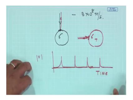
All we do if a shaft is rotating we shine a light. As you know the light speed is very, very high 3 into 10 power 8 meters per second.
