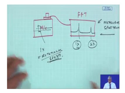
If I put a transducer to measure the vibration and if I do an FFT of it fast would it transform I will see certain peaks. So, this could be 1X or this could be 5X. So, you see this x is related to the rotational speed if there is a shaft here. So, when I am doing a fault diagnosis I will be looking for 1X and 5X frequencies in my measured spectrum measured spectrum.
