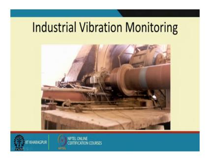
If you see the industrial scenario of vibration monitoring for example, this is a part of a cement plant, wherein this is the torsion shaft which is being driven from a speed reduced gearbox and there is the pinion gear here which is matched with the ring gear of the kill.
