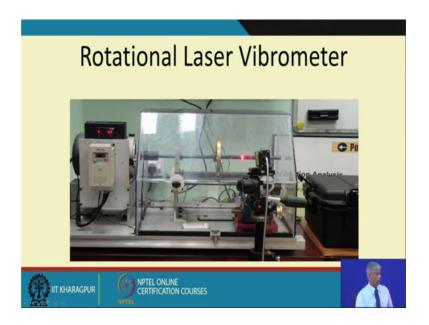
And here, if you see there zoom picture here you will see 2 dots this corresponds to those 2 laser beams which are being put on the shaft. So, you can very easily measure the speed and actually in many condition mounting. It is not the mean speed it is the fluctuation speed and this fluctuating frequency are because of the load torque, which is because of the defects I say defects or any conditions.
