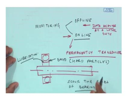
So, this monitoring, as I told you right in the beginning can be 2 methods, one is offline, another is online. So, in time monitoring what we have we have permanently mounted transducers. offline they could be permanent, but data analysis is done at a later date. So, for critical machines one has to do online monitoring because in real time one gets to understand what is the condition of the machine component?
