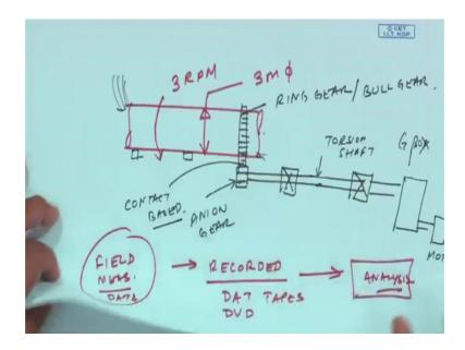
So, I will if I was to draw this one view, which is rotating about 3 RPM very slow RPM and this diameter is about maybe 3 meter and. So, if this is rotating there are sort of gear and of course, these are all supported on bearings cycles. So, if I have a ring here all around it and on to this I put a pinion gear which is driven by this is put in the bearing long bearing. and then there could be a gearbox which has been driven by a motor.
