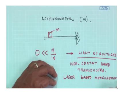
This was monitored by what is known as an contact based measurements and when we talked about contact based measurements, you know this accelerometers have a mass some mass. Now, imagine if I am measuring the vibration of a very thin structure and if I put a heavy transducer of some mass n the transducer mass is going to affect the dynamics.
