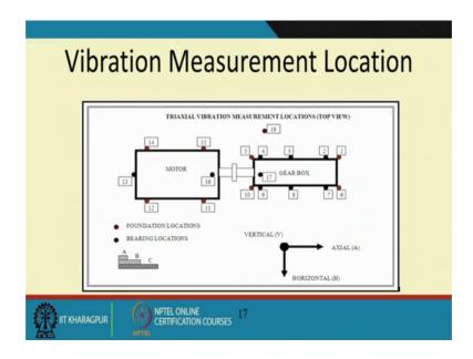
These are some of the locations where we need to put the transducers because everybody needs to know where do I put the transducer. When you know I am doing a vibration monitoring it is usually the bearing locations or the foundation locations and..
