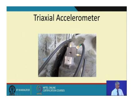
This is the bolted onto which I have glued my block onto which I have screwed this tri axial accelerometer. So, this is a good practice to have in your kit when you are going to do vibration based measurements to carry some of these mounting blocks with you. And
