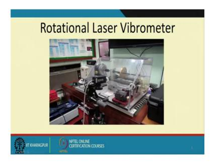
This is another view of their rotational laser vibrometer you know and this these systems are very expensive compared to the traditional linear based vibration measurements. Using accelerometers or optical encoders nevertheless they are advantageous because they are non-conducting and you can measure them from a distance.
