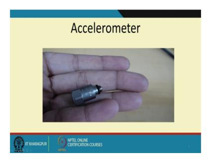
So, you get an idea of how big or how small this piezoelectric accelerometer is, but something regarding this charge as you know this charge which has been produced by this accelerometer will decay with time.
