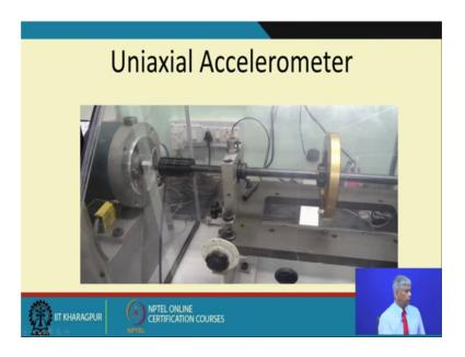
This here you can see an uniaxial accelerometer, being put in a rig to measure the vibration.
