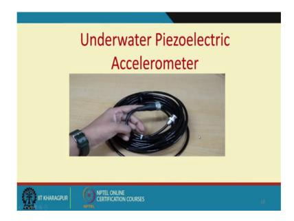
So, to measure the underwater vibrations we also have underwater accelerometers you will see this is the accelerometer here and again they have long cables integral with the accelerometer and then will it have an output which are used. So, today CBM does not mean only measuring machines you know which you see in a in a shop floor underwater measurements are being done to find out the impact of you know underwater piling noise.
