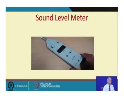
A microphone is put in a sound level meter wherein we can measure, there you can get a digital display or the sound level being measured.
