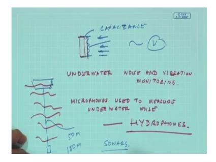
So, this membrane would vibrate because of the sound pressure. So, the capacitance would change and then we will have a corresponding voltage and then of course, in piezoelectric microphones we have a piezoelectric layer put here and such.
