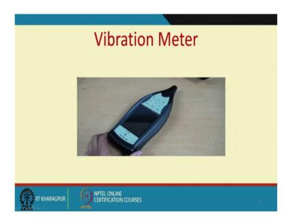
I can get either the velocity spectrum or the displacement, we could put it in a vibration meter. So, that either I can see the vibration spectrum in a vibration meter. I could see the RMS value, I can see the mean value or even I can see the vibration spectra a spectrum.
