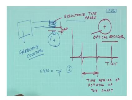
Sectional view of a shaft with a key which is rotating now suppose I put a simple electromagnet and every rotation what happens this gap is going to change. Now, this is an electromagnet or a reluctance type probe. So, what happens in time every rotation? Once the keyway just comes below the reluctance type probe the gap is going to reduce. So, I will get a voltage so, the time interval between 2 consecutive gap is the time period of rotation of the shaft.
