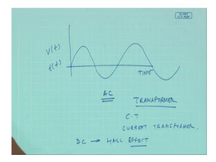
Relate to the voltage or the current, if the voltage is varying you see I can have a transformer either by a step down or a step up. So, this is known as CT coil current transformer coils and then we can measure the voltage, but even if the signal is DC.
