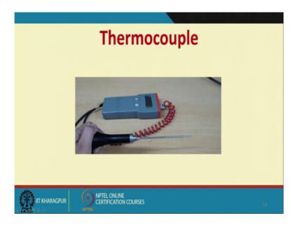
We will discuss this when we talk about electrical machines such transducers are also available thermocouple. Because of 2 metals kept at a different junction. Because they
