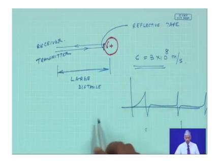
So, we will put a reflective tape so, if there is a beam which is going on same instance I will get a beam back. So, again so, the problem with the advantage of optical probe is they can be from a large distance. So, it takes only a fraction of a second because you
