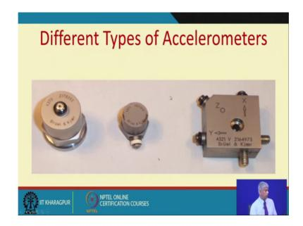
So, as you know vibration is very directional. So, the sensing element the piezoelectric crystal which is put inside this different accelerometers her also have direction to which they are most sensitive. And this is an uniaxial accelerometer and by the way this is this is about you know this diameter is about around 15 mm in size about a 50-paisa coin size.
