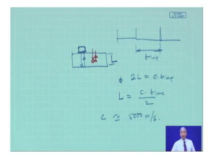
From and because of the impedance variation between surface there will be reflection back. So, the time taken between the incident and reflected back this is the time. So, and this distance is l. So, I know l because it is going and coming twice l is equal to C by t. So, I can find out L is C t times 2 and C for ultrasonic.
