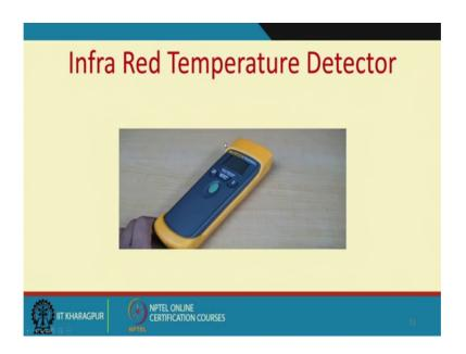
We have also infrared temperature detectors where you talk about thermal graphic. We will see how the infrared energy emitted by a surface can be measured as function of it is absolute temperature to the power 4. And then we can measure the temperature of the surface which is radiating this infrared energy.
