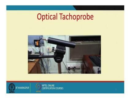
Because lot of optical tacho probes are also being used wherein we have a surface which is rotating.
