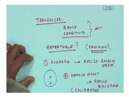
Now, any transducer which we measure; which we buy from the market has some features in it, most important being, it is range sensitivity, we need to know these quantities. So, that the mechanical quantities which we are measuring can be equally or can be represented with an equivalent electrical value or a voltage value.
