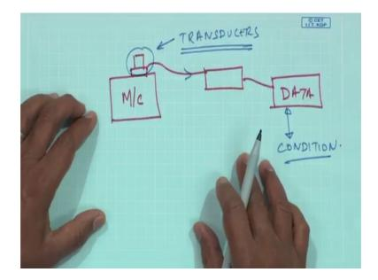
And as you know by now that in CBM, I have a machine on which I put a transducer and I have a signal conditioner and then get some data. So, on analysis of the data, I infer that machines condition. So, when you are talking about transducers we will see that; what is the possible errors while measuring using a transducer and how we can avoid it ok.
