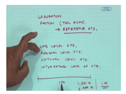
Which need not be used daily, but you know any transducer which goes out of the field can be brought back to the laboratory or to the tool room to check the values against the reference standard kept locally in that place because as you all know.
