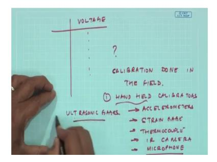
So, always it is good to have a calibration done in the field by there are certain hand held calibrators for accelerometers, even for strain gages, there could be some sand bridge calibrators strain gage, even for I would say hand held or portable caliber for thermocouples we will talk about this later on from I r cameras for microphone.
