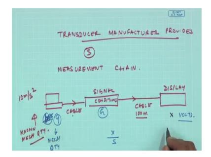
And now question is if I have a measurement chain, wherein I have got a transducer, I have got signal conditioner, I have got some cable and then I have a display. So, this in this cable also, there could be some attenuation. For example, if you are talking about a long cable, now you are measuring the condition of a popular bearing in a large ship where the cable could be about 100 meter long.
