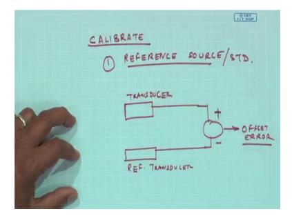
So, by calibration, we can remove the bias error. Now how do I calibrate? So, there are many methods of calibrating one is we have of a reference source or a standard where we will compare the results from the transducer and the reference transducer.
