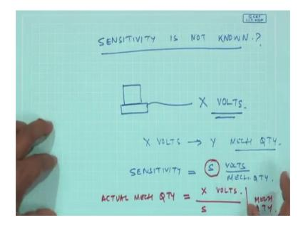
Suppose the sensitivity is not known, how do I do or what do I do? Suppose, I have a transducer, I have put on a machine, I get some X volts. Now this X volts corresponds to some Y mechanical quantity, right. So, unless I know the sensitivity. Sensitivity will be some you know S volts by mechanical quantity.
