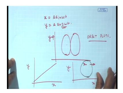
You would have seen if I compare known signal say for example x is equal to A sin omega t and y is equal to A sin 2 omega t and if I plot x versus y we will see that there will be loops and so on. So, if one signal is known the other signal can be founded and so on. This kind of orbit plots we have seen, if x is equal to y I will get a straight line like this, if x and y are 90 degree phase difference I will get a plot like this.
