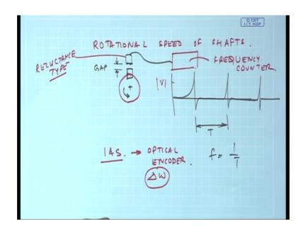
So, for example, a shafts is rotating essentially a shafts has a key shafts is rotating. So, if I put a probe here or a reluctance probe, which senses the gap between voltage produced is proportional to this gap here. So, every rotation of the shaft I am going to get a pulse. So, this again the inverse of the time taken or just by having a an f is nothing but 1 by T, just by having a frequency counter I can get the rotational speed of the shafts.
