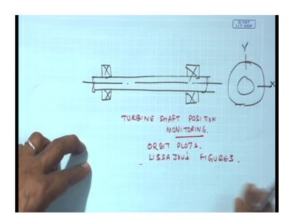
So, this kind of orbit plots we have seen are helpful in finding out the displacements or amplitudes in a shaft, so which is rotating supported on bearings and if I look at this end view here, if I measure an x here with the transducer y with the transducer I can see if x and y are same or different my ploy just plotting the orbit plot. So, physically for turbine shaft position monitoring such plots are used orbit plots or they are also in the one of lissajous figures.
