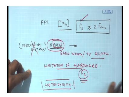
But question is when we have a signal so for example, 10 gigahertz for example, a very very high frequency signal which is not true in mechanical systems, we do not have such signals in mechanical systems, but perhaps some electromagnetic waves like you know
