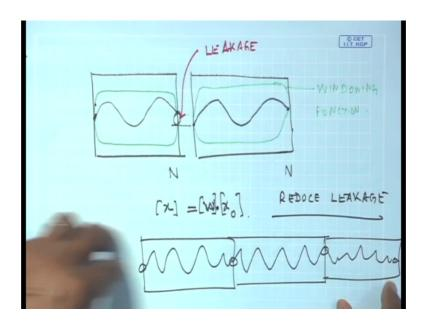
Now another possible error in FFT is what is known as a leakage error see for example, when we assumed or did FFT on a window block, we took a window of N data points, now signal like this the next signal would assume. So, if I bring this signals closer I will have maybe this kind of a gap, so this is what is known as a leakage.
