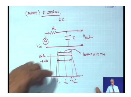
Of course, another technique of finding out frequency content of signal is through filtering. I will name it as analog filter, so the combination of RC circuits, I can get some output depending on R and C I can design filters and I can have series of such filters and then for any signal I can have a filter, which will have certain bandwidth and then this is the floor and f upper I will have a central frequency and this is 0 d B.
