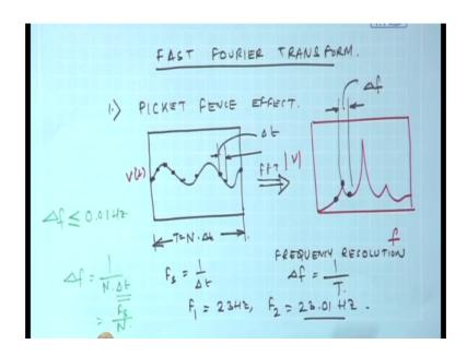
Of course, the next technique is FFT. By now we have you all must be knowing for this fast Fourier Transform is I will come to this filtering and heterodyning a little later, but let me tell you 2 most possible errors in FFT because whatever be it. My purpose is to accurately estimate the frequency contained in a signal and the amplitude at that corresponding frequencies.
