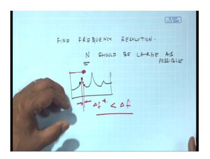
If my sampling frequency is fixed F s I can only increase N so that means, to have fine frequency resolution your N should be large as possible. There are of course, there are limitations why N cannot be large because of the memory requirement because every data point requires a storage space or a memory space. So, I cannot make N very large because that will be limitation of my storage space.
