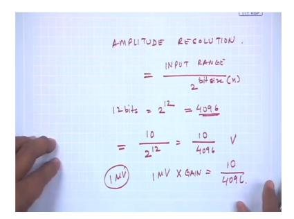
So, as you recall amplitude resolution is nothing but the input range by 2 to the power bit size which is denoted as n. So, this is a 12 bit data acquisition system, so the possible values are 12 bit means 2 to the power 12, so this becomes 4096 if I am right here. Now,
