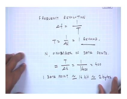
So, if the time is large my frequency resolution will be smaller and here we have asked that it required delta f is 1 hertz. So, T is become 1 by delta f so T is 1 second. So, basically 1 second of data sampled at 400 hertz is what my data acquisition system needs to acquire in 1 block.
