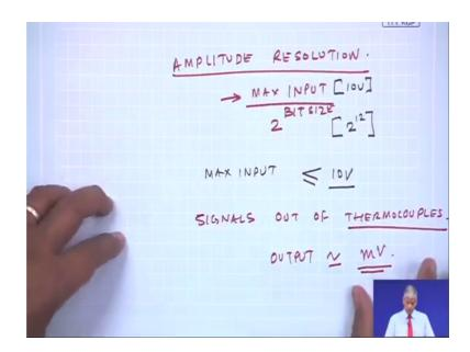
So, couple of takeaways from this numerical example, one is how could I have made the amplitude resolution small enough, so that it was able to sense I could have, because if you see this is the input, maximum input right 2 to the power the bit size, so to make this quantity smaller I could have reduced maximum input by reducing the input range and here, this corresponded to 10 volt in our case and here this corresponds 2 the power 12.
