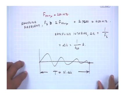
So, the signal frequency the maximum frequency of the signal F max is 200 hertz. So, from my Nyquist sampling theorem the sampling frequency should be greater than equal to twice F max. So, the least would be 2 times 200 that is 400 hertz, so my sampling
