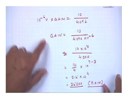
So, 1 microvolt is nothing but 10 to power minus 6 volt times again should be equal to the 10th power by 4096. So, the gain would be 10 divided by 4096 and 10 to power minus 6, for the sake of computations, 10 in 10 to power 7 by if I write this as 4000, so 10 by 4 times 10 to the power 7 minus 3, so 10 by 4, 2.5 times 10 to the power 4, 25000. We require such a high gain, to sense 1 microvolt in such a data equation with 12 bits.
