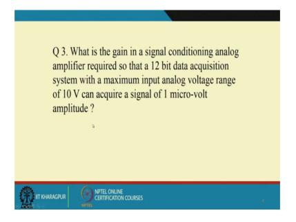
Now, let us look into the next problem. Now what is the gain in a signal conditioning analog amplifier required so that a 12 bit data acquisition system with the maximum input voltage range of 10 volt can acquire a signal of 1 micro volt amplitude. The second problem related to the signal frequency and this one relates to the amplitude resolutions.
