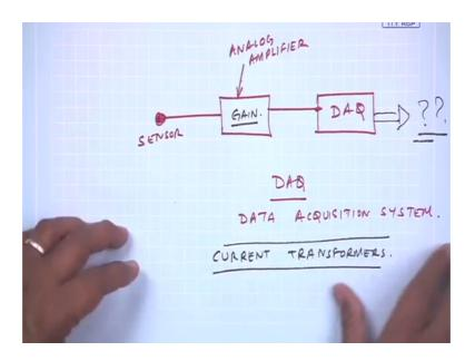
In such systems, we can always between the sensors, I can put an analogue amplifier and of course, then I have my DAQ system. Well you know DAQ the way I am writing is its, in brief for data acquisition system and of course, then you will have the right voltage out of this, so depending on the amplifier I can put some gain.
