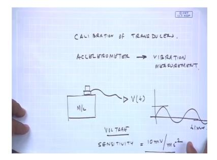
We will see later on that accelerometers are used for vibration measurement, but as you would have seen when I have a machine if I put a transducer I get some certain signal voltage as a function of time, looking at this voltage level depending on the sensitivity of the transducer say for example, this sensitivity is 10 millivolts per meters per second square there is a typical sensitivity of an accelerometer.
