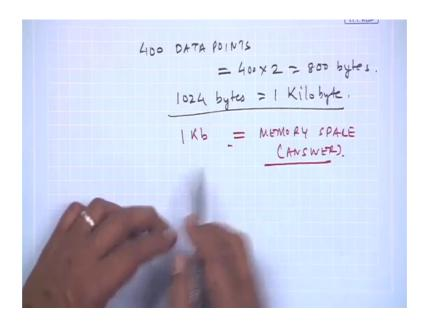
So, since I have 400 data points, the memory would be 400 times 2, that is 800 bytes. Well, so know since the memory blocks are available in only 2 to the power something, so the closest number of points would be 1024 bytes, this 1 kilo byte.
