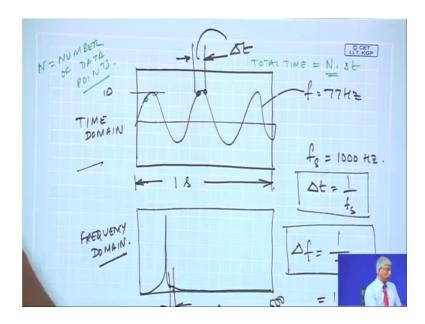
So, to begin with I generated a sine wave of amplitude 10 this are frequency is 77 hertz, where my sampling frequency was 1000 hertz. So, delta t is nothing, but 1 by f s so, at every 2 points this is my delta t. And this I took for n is equal to 1000 and this was only for total time was 1 second. Now once I went to FFT I plotted till 500 hertz, and the spacing just was this is here delta f. So, delta f is nothing but 1 by total time.
