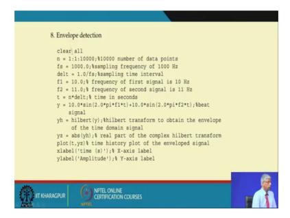
Now, I will move to the next. So, you can do an envelope detection because whenever we have the case of amplitude modulated signal so this is an amplitude modulated signal here. So, I will just do an Hilbert transform of this signal, and then absolute value of the Hilbert transform actually gives the envelope of that signal ok.
