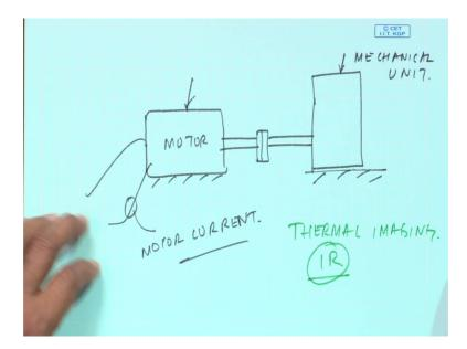
I was just telling you in motor current signature analysis is any electrical motor, which is driving. This is a motor through a coupling which is driving a mechanical unit; so, if a fault occurs in this mechanical unit; I could understand by analyzing the motor current. We can of course, understand the condition of the motor; we can also understand the condition of the mechanical unit. And that is what we will be covering in motor current signature analyzes.
