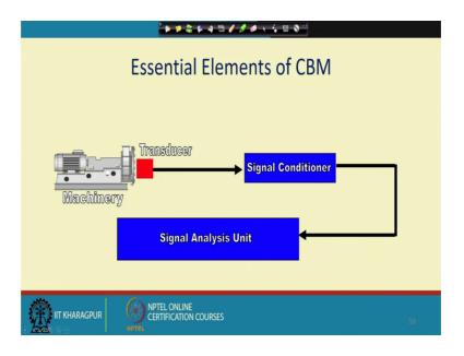
So, in the CBM we have machines, transducers, signal conditioners and the signal analysis unit; so, we will be covering this in details.
