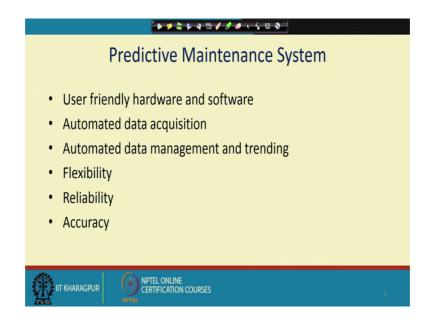
But a predictive maintenance system today; has a lot of hardware in it, hardware are essentially the transducers and then there has to be a automated data acquisition system so that all the sensors, all the signals from the sensors coming to the system and then there has to be a software. The same system today is being in the steel plant, the same one could be used in a paper mill, in a cement plant, in a ship, in an aircraft.
