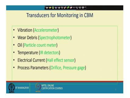
And as I have told you in CBM or condition based maintenance, all these written in black vibration, wear debris, oil, temperature, electric current, process parameters; these are the mechanical parameters which would change with machines condition and we need to put transducers in place to measure the condition of these signals. And then we will be talking about these transducers or equipment later on, when we talk about instrumentation.
