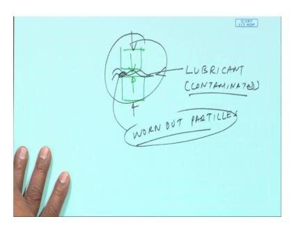
So, we put earlier of lubricant; so because of this forces particles will get worn out and get deposited and the lubricant also gets contaminated. So, the level of contamination of the lubricant and the composition of these worn out particles; gives us some clue as to the condition of the machine. And this is what essentially is done in the wear debris analysis, these are the contaminants which could be analyzed where chemical composition known.
