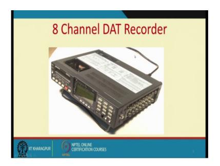
Well this is a view of an 8-channel analog that recorder. If you will see here we can have 8 analog inputs, and 8 analog outputs. Of course, the digital conversion is done inside. And by 8 channels I mean 8 inputs can be taken in simultaneously. And then it this comes with a digital audio tape.
