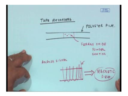
Basically, the tape is nothing but a polyester film on which it is coated with some ferrous oxide powder coating. So, if I have an analog signal given into is an iron core. This will create magnetic field, the variations in this magnetic field will be proportional to the variations in the signal. And because there is a magnetic field, the ferrous oxide will be accordingly because of their hysteresis will record this magnetic field which has happened because of an analog signal.
