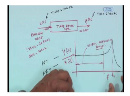
You record with an random noise; that means, for example, if you are talking about an audio frequency maybe from I mean, a though it is 20 hertz to 20 kilohertz. You it is no harm if you give a signal from 0 hertz to 20 kilohertz. So, this is my input signal.
