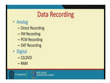
One is a direct recording or a frequency mode listen recording or a pulse code recording or a dat recording. We will see how these are done. And of course, today if you have digits. We can do them in digital recording; that means, we have nothing but a memory
