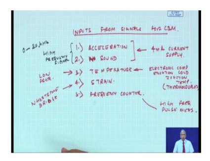
One is of course the acceleration. Another is maybe noise or you know size or sound, temperature. Then we have a strain, maybe a frequency counter. So, typically one would come across such input signals. So, we will cover about this later on, some of this sensors require a 4 milliampere current supply to drive the sensors. And as you will see
