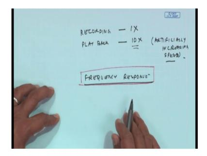
This was the earlier provisions were there in the tape recorder, because many of the analysis equipment either did not have a very loop or lower frequency response. So, they had to record at a higher speed, and played back at a recorded of speed and played back 10 times and then of course, you can do the other way also. So, you could do some amount of frequency scaling by such varying the speed between recording and playing back.
