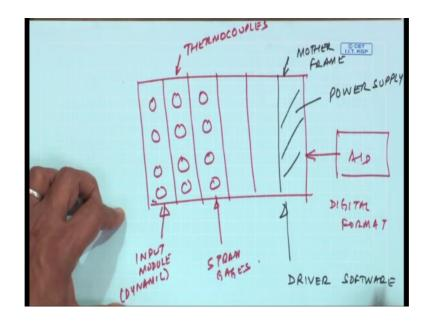
And if you look at the view of any data recorder the input model is what matters. So, input model 1 2 3 4 and there will be some connectors like this and so on. So, this is an input model. May be an input model for dynamic signals for all terms of thermocouples, for maybe strain gauges and so on. So, all of these go into their corresponding A to D, which is inside this and then they get recorded you know digital format.
