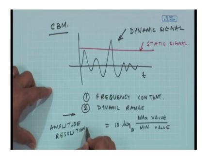
This is an example of a dynamic signal as opposed to maybe static signal. So, if you consider the dynamic signal, you will see that there are few important features of dynamic signal. One is the frequency content, other is the dynamic range or a dynamic range, I mean what is the in a logarithmic scale 10 log to the base 10 of maximum value to the minimum value present in the signal.
