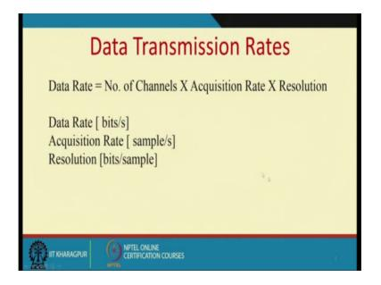
Because you recall this which we discussed during our class on data acquisition that the number of channels is nothing but the number of inputs into the system, acquisition rate is samples per second and if you recall to avoid aliassing I have to acquire these signals at a rate where the frequency is at least twice that of the maximum frequency contained in the signal. And every data requires certain bits.
