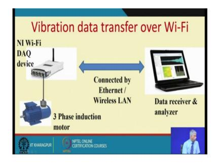
So, I will show you an example where even we are doing a vibration data transfer over Wi-Fi, you know in the in the laboratory. So, what we have here is a motor. We have an accelerometer which is or a sensor which is used to measure the vibration. And this is an data equation device which can take in frequency here 4 analog inputs. And it acquires it, and then it transmits it over the Wi-Fi.
