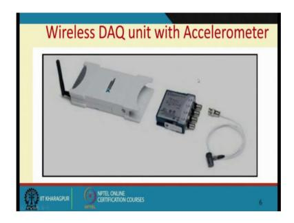
It connects at the machine and through the cable, but then this entire unit is kept at the machine unit, and then we have an Wi-Fi transmitter which transmits the signal.
