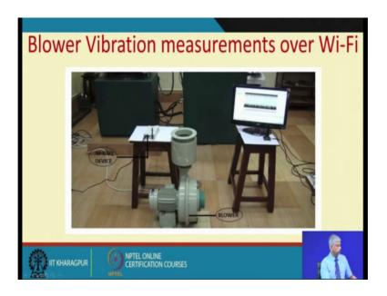
In the laboratory we have a blower; it is actually 3 phase motor. And if you see here there is an accelerometer which has been mounted on the blower. And this is the Wi-Fi device which has been put here. So, all the cable goes in here. And on the blower was run at a certain speed, this data was acquired and it was transmitted.
