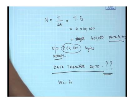
N is nothing but T divided by delta T or t times Fs. So, that is 10 times 40,000. So, this is 80, 800. Sorry, sorry 400,000 data points. And as I was telling every data point takes 4,000. So, the total number of space is 800,000 bytes the memory require is so much. So, I require 8,000 of bytes and if I want to send it at a rate of you know whatever is the throughput.
