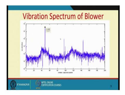
And then we analyze the vibration spectrum of the blower. See if you see here the wireless captured data in the frequency domain. Once we did the FFT you see here there is a frequency of 48.38 and what could this be this was an induction motor.
