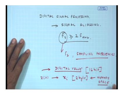
So, if you recall the class on computer data acquisition, I had mentioned to you about the condition of signal aliassing. So, to avoid signal aliassing we have to have the sampling frequency which is greater than equal to twice of f max. So, the type of the signal when we talk about acoustic emission, greater than 1 megahertz or 2 megahertz, when we talk about temperature signals less than 100 hertz.
