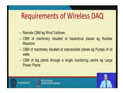
So, just to recap you know we will discuss this, but then what are the requirements of a wireless it is helpful to remote condition-based monitoring of wind turbines. Imagine a wind turbine which is you know there in the high seas where we it is just not possible to lake cables some signals be acquired through cables inside nuclear reactors inside you know pumps of oil wells etcetera. So, these are good candidates where in the wireless data acquisition can be done in mines and so on.
