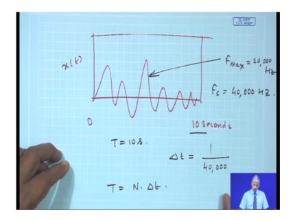
And if you for example, I have. A signal which is happening at time and this is 0; this is 10 seconds some signal xt. So, if I want to capture 10 seconds of signal where capital T is 10 second. And imagine if this was maybe a acoustic signal. So, the maximum frequency here f max is 20,000 hertz. So, at least my sampling frequency should be 40,000 hertz. Now, that means, your delta T is 1 by 40,000, right.
