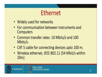
We also use the Ethernet once the data is in digits and of course, we have the CAT 5 cable connecting devices we have the wireless Ethernet and so on. So, today is world in a bit machines computers mobile devices we need faster ways of transferring digital data through this protocols which are available and then we can do our processing and make an analysis.
