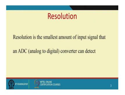
And then another quantity is resolution, what is the minimum value the signal can be sensed I will give you an example here, because see all the signals which are digitized I have an analogue domain and then I have a digital domain.
