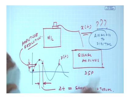
What do we understand from this as signal xt and. So, that is why we have on a nice module of signal analysis, but to do any mathematical signal analysis or DSP, I need to convert this signal from analogue to digital.
