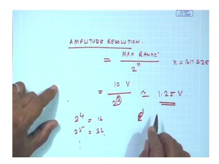
So, this amplitude resolution which I am talking about is nothing, but the maximum range by 2 to the power n where n is a bit size, if maximum range of 10 volts and 3 weight we saw this as 1.25 volt.
