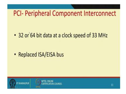
And then PCI a interconnect it is a clock speed of 33 megahertz, which is replaced the ISA EISA bus.
