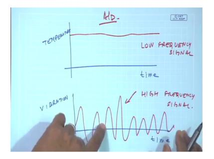
Temperature signals do not change so rapidly unlike a vibration signal vibration signal could be changing very fast, but a temperature signal is very slow slow. So, this is a very very low frequency signal, and this is a visually high frequency signal. So, the data acquisition system A to D converters, for temperature recording conversion is actually I can have a low frequency signal sampling frequency. In fact, they are much much
