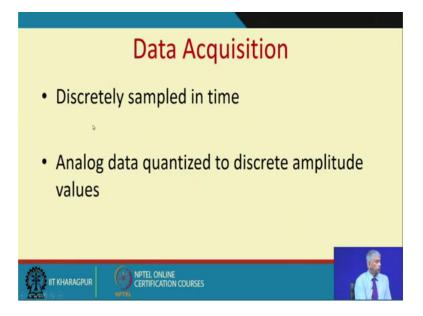
So, this is what we are going to focus on introduce class. So, data acquisition is values which are discreetly sampled in time, discreetly means there is a definite time interval between the signals. So, this delta t is known as the sampling interval, a device hardware
