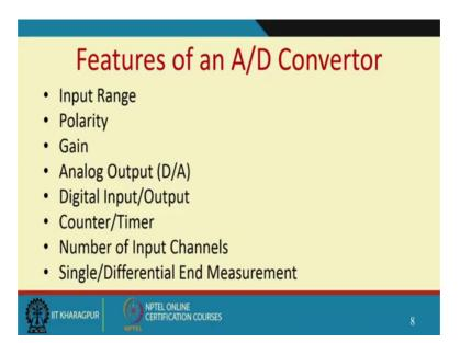
But then there are few other features of A to D converter, one is this maximum input range its usually you know 0 to 10 volts polarity, sometimes you know whether they will be bipolar or unipolar gain sometimes some of this data acquisition units the least sensitivity or amplitude resolution is so low, that even a thermocouple signal giving few millivolts cannot be sense.
