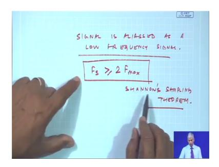
So, signal is aliassed as a low frequency signal so in fact, there is a theorem which says your sampling frequency should be greater than twice of f max to prevent signal aliassing. So, this is the Shannon's sampling theorem. So, to prevent signal aliassing we have to do this.
