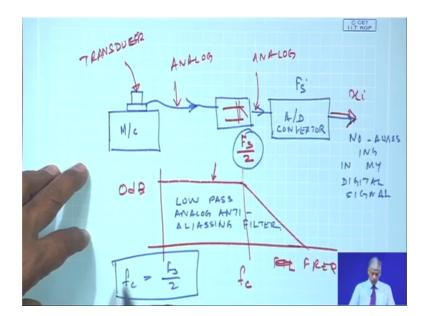
But the question is many a times in this A to D devices, I have my machine here and I have a transducer, I am giving an analogue signal and I have one A to D converter, which comes in the market the sampling frequency and then I have to put some device here so
