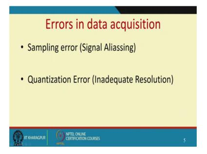
So, the errors because of data acquisition one is the sampling errors, which we discuss is known as signal aliassing and other is the quantization error because of the inadequate resolution I will explain it through a better diagram here.
