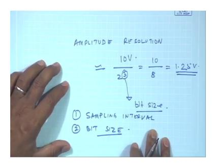
So, store this value. So, this amplitude resolution is nothing, but your total voltage. So, in our case 10 volts divided by 2 to the power 3, 10 by 2 to the power 8 is 1.25 volt. You see this bit size plays an important role in the resolution of this A to D converter. So, one thing that keep in mind, one is the sampling interval I will give an example of the sampling interval and other is the bit size apart from few other things.
