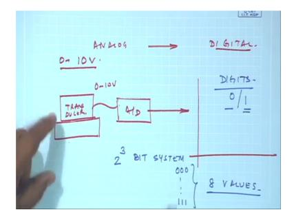
So, in analogue domain I have a analogue voltage may be from 0 to 10 volts this is my transducer output. So, in transducer gives me maximum value it can give to 0 to 10 volt analogue signal.
