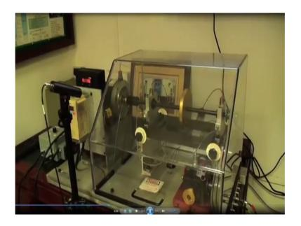
And let me show you this. If you see here this is an rotor rig, wherein we have put transducers in, explain you know if you see here. There is one in the x plane and one in the y plane. And these transducers are for some other measurements which we are doing in the laboratory, and this is a rotor which is supported on 2 bearings driven by a motor at a constant speed. And these are the 2 transducers, measuring one is measuring x and other is measuring y.
