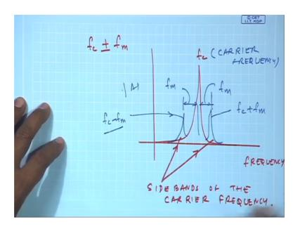
So, if I have a carrier frequency fc in the frequency domain, I will also have amplitudes at frequencies of fc plus fm and fc minus fn, some amplitude of this amplitude modulated signal. So, this has the name so this is the carrier frequency and these are the modulated signal which are known as you know spaced at distance of fm. So, on other side of the carrier frequency, so these are known as side bands of the carrier frequency ok.
