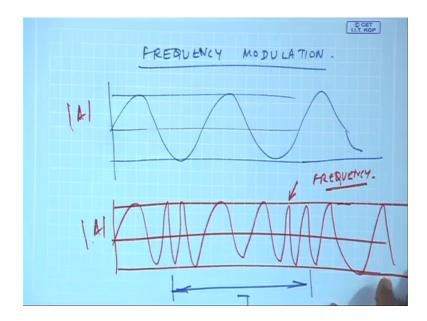
But another type of modulation which is known as the frequency modulation, see if I have a sin wave; what I could do physically see I could increase the frequency decrease the frequency and then I could have I will have another information being conveyed by the same signals.
