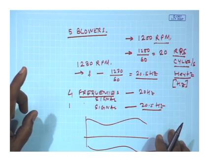
Suppose you know plant I have 5 blowers and each of 1 of them is supposed to run at 1200 rpm. So, in rps or cycles per second this will be to 1200 by 60 that is 20 rps or cycles per second or hertz represented as Hz. So, in many of the case places you will see units of frequency given in either in rpm rps cycles per second cycles per minute hertz.
