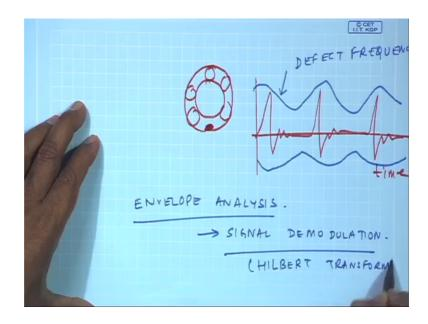
If there was a defect here in the race and every time, every revolution this defect would give rise to a pulse and this could be amplitude amplified during load.
