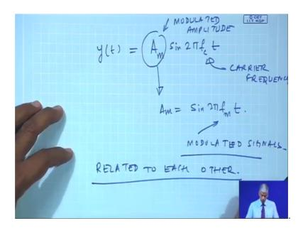
If I also write the equation of this signals say an amplitude modulated signal yt, in general is a m sin 2 pi fc t where m equal to another maybe sin 2 pi fmt.
