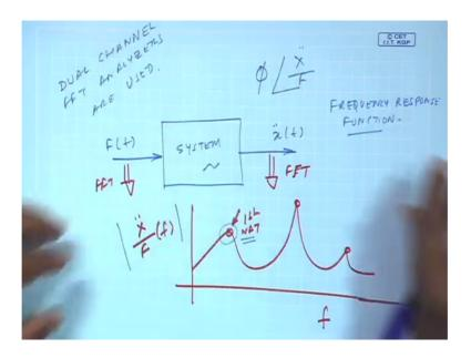
I can always do an FFT of this, FFT and get the plot f nothing but either x dot lot by f or occurred in the frequency domain. So, this corresponds to the first natural frequency and so on. So, there will be a change and this is nothing but the amplitude, and there will be also a phase angle of this and we have seen in vibration and natural frequency is how the phase angle changes by 90 degree.
