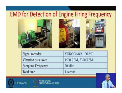
This is an example which we thought ill introduce you from our lab this is an engine single cylinder engine which is being loaded by a dynamo meter, and this is an
