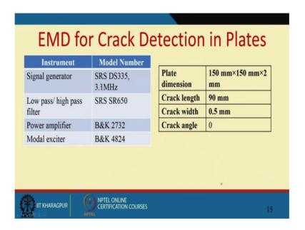
So, this signals now already did an EMD, a plate has dimensions of 2 mm thickness 90 mm is the crack length 0.5 mm is the crack width. And these are some of the instrument which we use to find out the crack.
