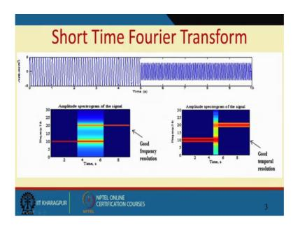
And then we will see the one such method is what is known as short time Fourier transforms. So, in short time Fourier transform what we do we break this time period into small packets of T. And do the FFT and then stand up together. But again, the problem is if I have a good frequency resolutions, I will need to have a by good I mean finer I need to have more time. And if I have more time I will have a poor frequency resolution. So, this policy exist because f is 1 by T or delta F.
