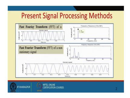
So, some of the signal processing methods, one is this fast Fourier transform if you here, this is a signal of one second durations. Amplitude from minus 5 to 5 here of course, you know this amplitudes meter second square. Should have been actually 10 by 4.997 is close to 5 that is within the limits of the measurement here.
