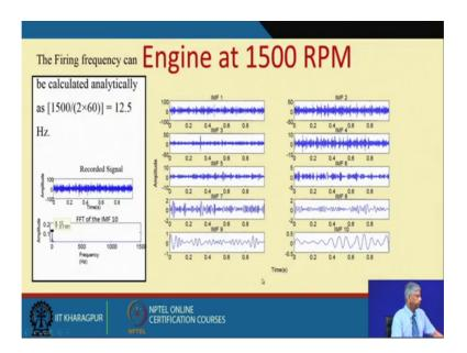
So, the IMF's of the engine was this is the recorded signal, through an EMD process the IMF's were obtain. We can see 1 2 3 4 etcetera. And the tenth IMF you see it gives a frequency close to the firing frequency of the engine. In that way even just in one second of data we can find out the 5 in the frequency of the engine.
