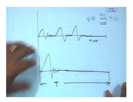
Now, when we do fast Fourier transform, certain time is being used to do this FFT, but the question is what happens in this time my signal is changing; that means, the signals quality has changed for example, I will give you another example illustrate. This I have an impulse and then there is nothing beyond it. And then if I have taken a total time signal of T; obviously, this is not true the signal is not repeating at many at any instance of time.
