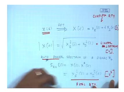
So, if I have a signal xt, if I do an FFT just saying I will get a signal xf, which is a complex number. So, it can be represented as x real plus x imaginary. So, the amplitude or magnitude of this Fourier coefficient is nothing but x real square plus x I square, these are all functions of frequency.
