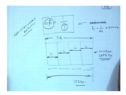
So, this is true. So, I can break up into different windows and do FFT, but then I will have higher resolutions of data F. So, this is what we see here a good temporal resolutions happens finer in the time, but poor in frequency or good in frequency more in time. So, we will miss the characteristics of the signal. So, this is a problem which people face.
