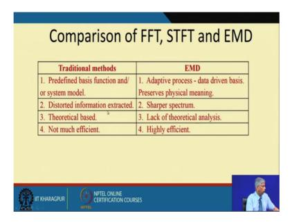
And this is more of an adaptive nature, and it is highly efficient compared to the traditional frequency domain analysis of FFT or STFT.
