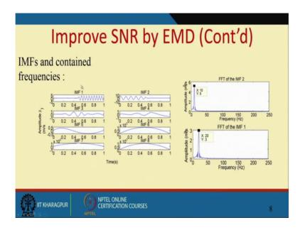
And then even see each of these IMF's contained a frequency. So, the actual representation of the frequency of the signals can be very easily done through EMD.
