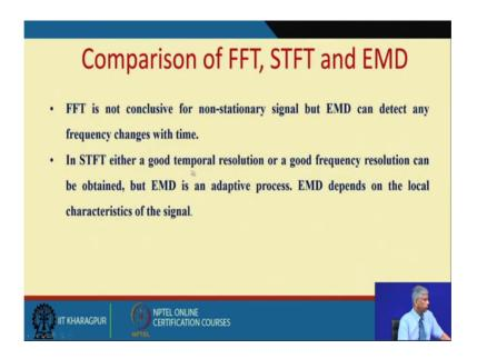
So, if I was to compare fast Fourier transform short time Fourier transform and empirical mode decomposition. So, a 50 is not conclusive for non-stationary signal, but empirical mode decomposition can detect any frequency changes with time. And in STFT either a good temporal resolution or a good frequency resolution can be obtained, but EMD is an
