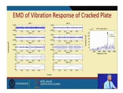
And if you look the EMD of a crack plate the response, I mean here the mobility is not being measured just by the response of a cracked plate IMF one IMF 2 in that same frequency as per the algorithm which I had told earlier. And FFT of the IMF 4 this the natural frequency has 732.2 volts.
