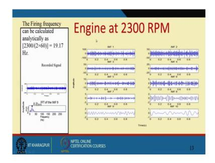
Same was also repeated at 2300 rpm and the engines firing frequency was 19.17 hertz.
