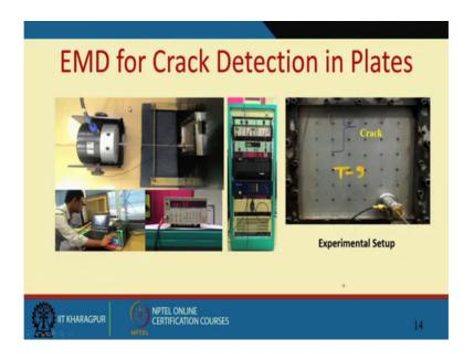
This EMD is also used to find out the cracks in plates. Where in a resistive. So, the reason I want I am showing you this now. So, that you get an feel of what kind of equipment later on will be using in condition monitoring.
