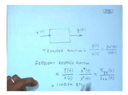
So, this is just the cross power spectrum between y and x and the auto power spectrum affects. So, this is again a complex quantity.
