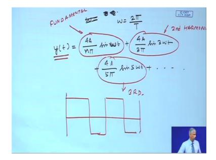
So, cosine square wave can be represented as 4 A by n pi and if you see here it is A n Bn sin n omega T. So, we have ans are 0. So, this will be sin n or omega T plus 4 A, where n is odd 4 a by 3 pi sin 3 omega t plus 4 a by 5 pi sin 5 omega t plus so on till finite terms.
