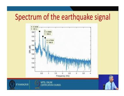
Of the earthquake signal, this is an frequency and you will see, this is the sound pressure level in decibel, in underwater, but you see a frequency of 0.3438, a very low frequency signal is predominant. This is characteristic of earthquake signals.
