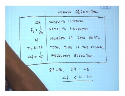
take the parameters delta t is nothing, but the sampling interval f s is 1 by delta t is known as a sampling frequency and in the number of data points t is equal to n times delta t is nothing, but total time of the signal delta f is equal to one by t is the frequency resolution.
