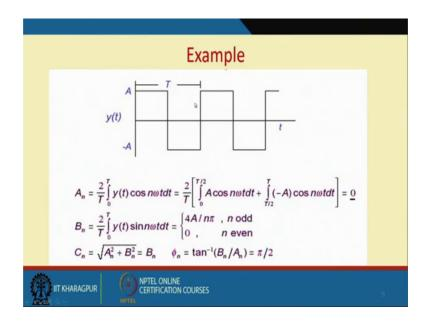
This is the example, wherein I have a square wave from amplitude a to minus a the time period t it goes up till infinite.
