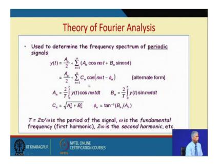
But we must have done this in our Math's class that if I have a periodic signal, I can represent it, periodic signal been y t, I can represent it as sums of sine's and cosines given by this expression, where A n is calculated by this expression 0 to T t is the time period of the signal and. So, on and B n is this and the amplitude C n is given by this and the phase is given by this expression here, where the first fundamental frequency omega
