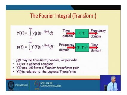
So, any signal yt can be represented, if I do this multiplication by e to the power minus g 2 pi f t dt from the time domain, I can go to the frequency domain or from the frequency domain by an inverse transform, look at the signature signs. Here I can get back my Fourier the signal. So, this is very important that I have a signal
