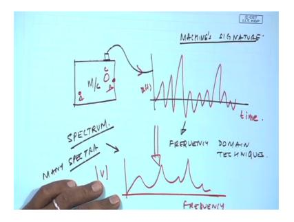
If I have a machine and I have put a transducer on some location did and there could be different components in this machine components A B C etcetera. So, it is this composite signal, which is going to come out in the time domain so; obviously, I am not able to use
