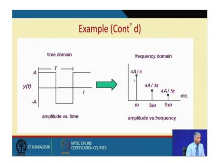
If I look at the spectrum, it will show as, at the fundamental frequency omega. It has an amplitude 4 A by pi, at this second harmonic. It has amplitude 4 A by 3 pi third harmonic by 4 A by 5 pi and so on and all the odd terms are there.
