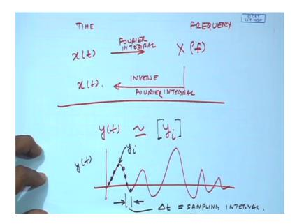
xt, I will do the Fourier integral, I will get the signal x f. This is in time domain and there is in frequency domain. So, this is the frequency and this is in time.
