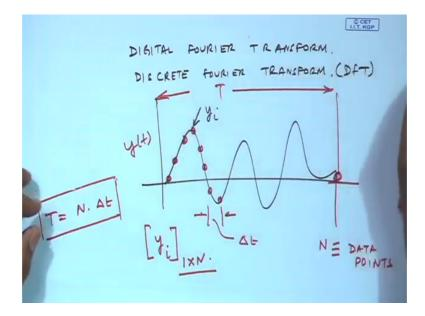
Digital Fourier transform or sometimes known as discrete Fourier transform. So, any signal DfT any signal, which is available to me I will, we will discuss about the sampling points, later on I can select through a mechanism yi for you know maybe n data points. So, this yi will be represent by an array series of number and this is known as the delta t. So, total time taken t is nothing, but n times delta t.
