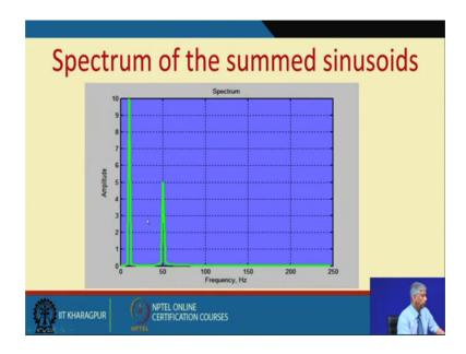
I can see that these two frequencies one of 10 volts 10 hertz and 5 volts 50 hertz gives rise to this kind of a signal.
