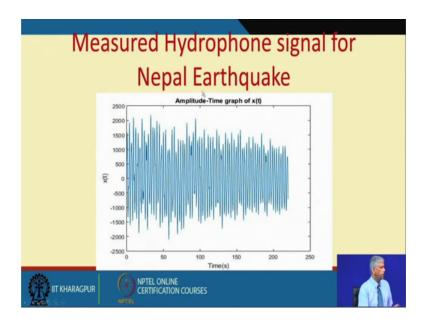
So, immediately the hydrophone captured this signal, because this is the time domain signal, time in 250 seconds and they found this signal, which is because of an earthquake and then they did the spectrum.
