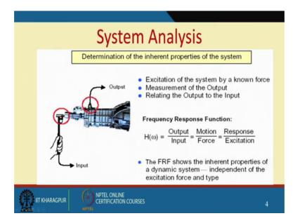
And for the sake of completion, I will just mention to you, mould dusting being done through, what is known as the system analysis? It is this output by input response by excitation. So, the frequency response function shows the inherent properties of a dynamic system, which is independent of the excitation force and type.
