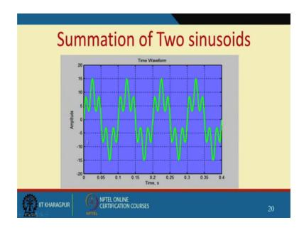
10 hertz corresponds to the amplitude 10 here in the spectrum but when I sum up two sines. It is very difficult for me to look at this time domain and tell what are the frequencies and what the amplitudes, but then if I go to frequency domain I can say well, that sin signal which I showed you here, basically consists of a 10 hertz 10 amplitudes sines or 10 hertz 10 amplitude sin wave and 5 amplitude 50 hertz sin wave sum together.
