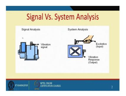
What is known as the signal analysis? So, basically I have a machine put a transducer.
