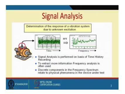
So, we find out in signal analysis, response of a vibrating system due to unknown excitations, if this excitation was known, I would have been having a nice machine, because I would have taken efforts to remove this excitation, but excitation occurs only, because there is a defect which has happened in this machine, because of various reasons could be poor design, could be you know lack of lubrication, could be wrong commissioning, wrong installation, wrong operations.
