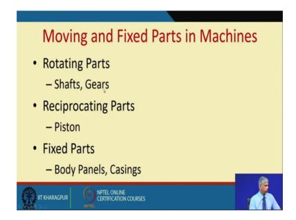
And as you know in any machine there are moving and fixed parts in machine rotating parts, reciprocating parts. So, all of these parts, when they rotate, they are responsible for generating signals, which are varying with time and it is this time varying signals, which we have to analyze in time domain in frequency domain in time frequency domain to find out what are the possible faults in the systems.
