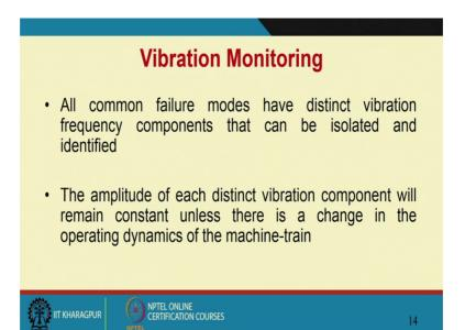
But then why do we do vibration monitoring because, all common training modes have distinct vibration frequency components that can be isolated and identified and that was the preamble wise vibration monitoring is so popular in CBM and in the next 1 is the amplitude of each distinct vibration component will remain constant; unless there is a change in the operating dynamics of the machine train, so you know if the there is no change.
