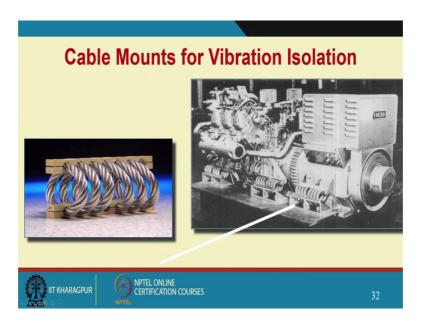
Cable mounts we discussed, cable mounts used in missile launchers ok.
