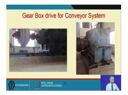
And this is just to give an example of on a conveyor system, there is a coupling here and this is on the concrete foundation or frame and the machine formation and this gearbox being driven by a motor driving the conveyer system.
