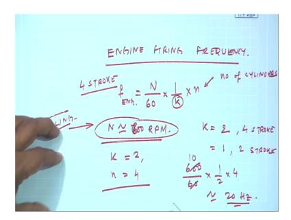
So, what is this engine firing frequency, in a nice engine suppose it is 4 stroke; that means, for every 2 revolutions I have 1 a power stroke. So, if they RPM of the engine is n so N by 60 is RPS divided by 1 by k, k is a factor k is equal to 2 which if it is 4 stroke and k is equal to 1 if it is 2 stroke times n, where n is number of cylinders and that engine.
