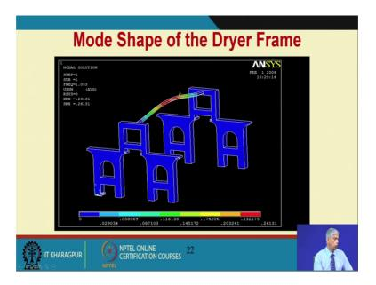
And then mode shapes of the dryer frame because this is an elastic model. So, we can find out the natural frequency of such systems and then you can find out that you need to avoid the natural frequency of this while you are in operations.
