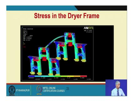
And then the stresses were determined using such finite element analysis, you can find out the dynamic stresses ok.
