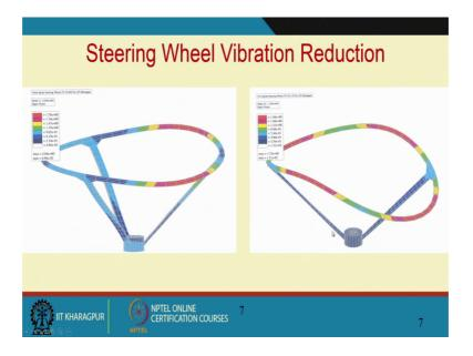
And then we studied this thorough a finite element model and found out the natural frequencies of the steering wheel, and we found out that the natural frequencies of the steering wheel was equal to the engine firing frequency.
