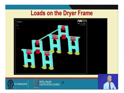
And we have done an find elements study to understand the loads on the frame. So, that in the vibrations called because of this dynamic loads are within the limits, other than the structural damage to the component.
