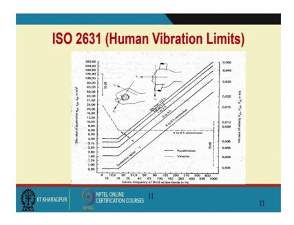
I was mentioning about that a jackhammer. So, there is an excuse me ISO 2631 human vibration limit standards as to at different frequencies, if somebody is having an exposure to 4 to 8 hours of less than half an hour, what is the permissible level in terms of velocity or in terms of acceleration ok.
