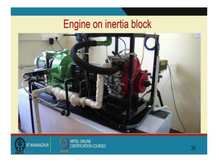
Another example is this inertia block because the objective is to reduce vibration, which is either getting transmitted or getting transmitted into the machine in a backhoe loader also again in the tractor.
