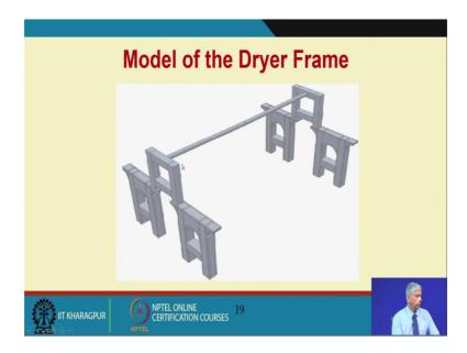
And we can do 4 because, if you look at the frame of the dryer and a paper mill there is a frame and the frames must not have resonance equal to the rotating speed of the paper mill rolls.
