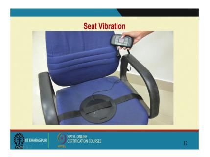
This is a seat accelerometer, this just to show you seat accelerometer can be strapped onto the seat and basically this has a accelerometer in between it and somebody's made to sit on it. So, if the seat is having excessive vibration this exposure limits can be measured on this human vibration analyzer. So, you can get the vibrations in the x y z and whether they are within the limits ok.
