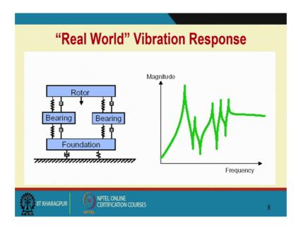
So, this is how one can play around with the natural frequencies designed to change the occurrence of resonance.
