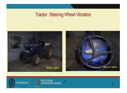
So, I will give you another example; so this is a tractor wheel steering wheel and the problem with this kind of tractor wheel was you know as long as soon as they started the engine, this steering wheel had an excessive vibration. So, our efforts at idea were how to reduce these vibration levels.
