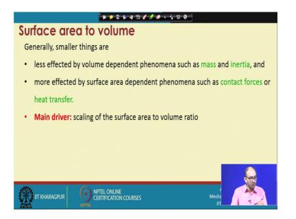
So, first thing is the surface to volume ratio. So, this is very important to understand because we have many components in the memes part also as well as the other components related to the micro machining operation, where we will understand where this surface to volume ratio is very important to understand.
