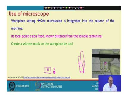
We will see how you can use those thing; for workpiece system one microscope can be integrated into the column of the machine. So, here it is a focal point; so our this is what is the focal point its focal point is fixed and known distance from the center spindle center line right. Suppose you have one system here; so, this is your spindle and this is your cutting tool and now you install one microscope here some location here rights and this located is.
