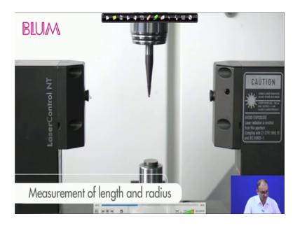
But you can use micro tool also. So, laser is coming from one location another it is a receiver. So, when it is coming here touching this location you can get the laser signal here and then you find out the length and the radius measurement then you can also if it is going up and up continuously then you can do measurement of a tip profile also.
