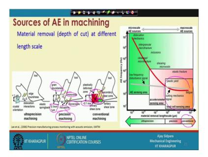
So, if you cover if you plot in terms of depth of cut now you can see here now this is the unconventional machining where you consider material removal length scale you consider as a depth of cut right. So, if you see conventional machining process when you talk about the depth of cut around 0.1 millimeter 100 micron or something we note that there are difference of one is the primary zone, this is the secondary zone this is the third tertiary zone shear zone.
