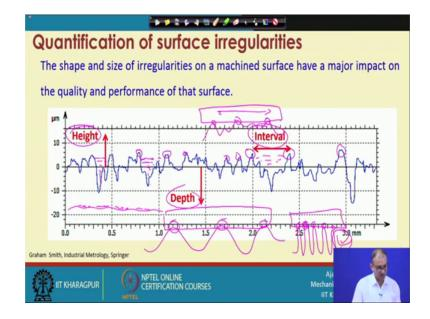
So, this is the routing graph which you can get which you can get from the surface profiler. The shape and size of irregularities on the machine surface have a major impact on the quality and the performance of that surface.
