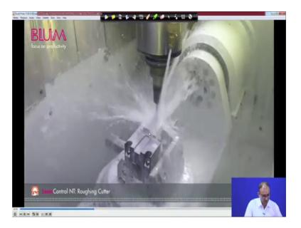
So, machining operation also after machining what you have to do? You to do measurement of the cutting tool whether the tool is wear out or not right. So, this is that laser part again; so, you put the laser here and then you do measure still it is useful.
