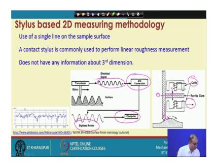
Now, let us see the stylus step; so, this is the stylus step you have surface this thing. Your stylus is moving up and down here and that will create a signal. So, this is the LVDT Linear Variable Differential Transformer and here right now it is exactly located at the center location.
