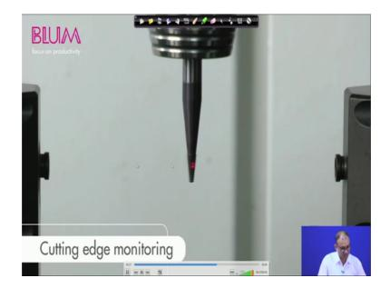
So, cutting edge monitoring now it is going one by one on the top surface and based on this laser transfer from one location to other way, you will get the edge monitoring also.
