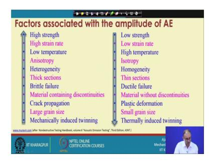
So, if you see the what are the factors which will increase the amplitude of the acoustic emission? If you see the high strength material then you will get a high amplitude high strain rate that is when your speed is very very high; you will get a high amplitude; low temperature if you increase the temperature material becomes soft, so, your signal strength will be low.
