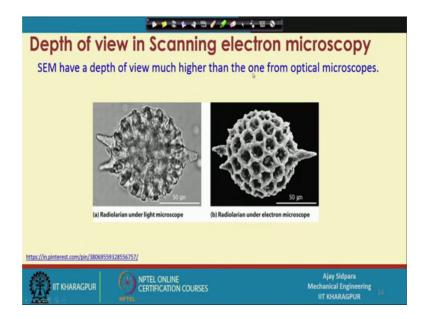
Here what is there? This is showing the depth of focus of that; that means, up to what depth you can actually do measurement; this is measured by the light microscope or
