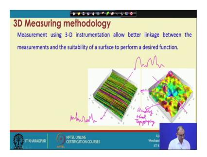
So, 3D measurement measuring, using 3D measurement allow better linkage between the measurements and the suitability of a surface to perform the desired operation. Now you can see the these are the two images; this is the topography of the grinding wheel.
