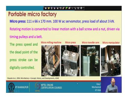
Now, press has this much area and hundred watt ac servo motor is used and you can get the 3 kilo Newton of load on the particular press and rotating motion because now here you have to press something. So, pressing getting that much amount of force is a very very difficult.
