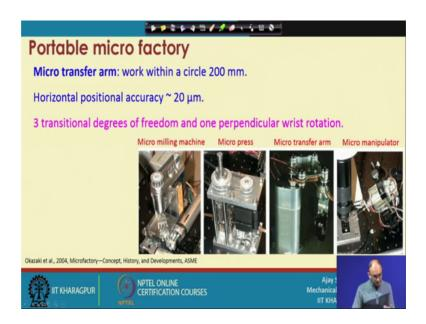
So, there are some micro control available which will do all this parameter settings micro transfer arm. So, it this is the third component it has a working old area circle in the 200 millimeter. So, it is very very large compared to the area of this. So, you can actually move one component from one machine to another machine very easily because you can see it is a twenty millimeter 200 millimeter is very very large.
