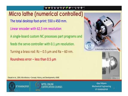
And roundness error was the less than 0.5 micron. So, this is showing much better result compared to the earlier case, but. So, this was the means; what we can say this advance version of the earlier micro lathe and this is the component which was processed here you can see the whatever the features, it was created because of the NC program you can give the curvature also, then you create a slot also.
