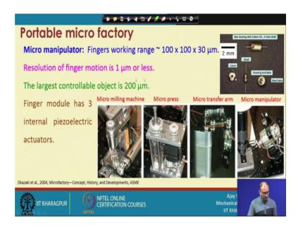
Now, coming to the last one that is a micromanipulator; so, it has a finger working ranges 100 by 100 by 30 micron. So, within that area you can actually give any component from the resolution of the finger motion is one micron or less. So, when you want to pin pointly, you want to target something, then you can go with a one micron. So, that is the advantage of one micron largest controllable object is 200 micron.
