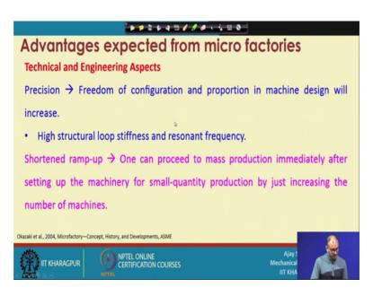
High structural loop stiffness and the resonant frequency; this is actually with the debatable things, here the stiffness is high in terms of the components only because smaller components are very difficult to deform in that way, it is there, but when you consider the loop stiffness of this particular part; that means, when all things are
