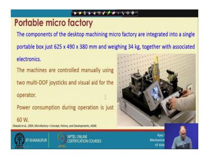
And if you assemble all this thing in a single part. So, this is the pool assembly of all that component now you can see that this are the this is the press is there then this is the manipulator is there then in the transfer arm then this is micro milling machine now once you do machining here what is happening that you cannot see anything by necked eye. So, here there is a visual look on instrument is available and you have a joy stick.
