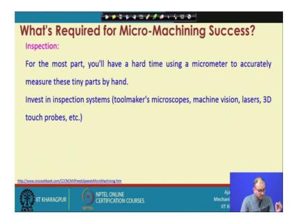
Inspection is very very important here because for the most part you have a hard time using a micro meter to accurately measure those tiny parts by hand. Because when you do micromachining your conversing machine you can use micro meter, you can use vernier caliper, or many things are there by which you can do the measurement.
