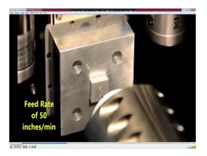
This is the work piece and this is the cutting tool and this is showing in the real life; that means, you are not using at high speed camera here. So, feed rate is 50 inches per minute, now you can see the way it is moving or it is doing cutting. So, it is showing in the real time.
