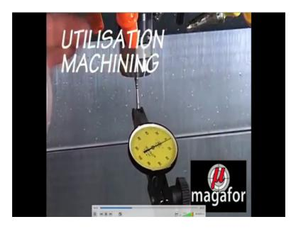
And this is you can see that it is showing what is the tool run out and this is the diameter of 500 micron. And you are cutting the pro machine this thing and this is at high speed.
