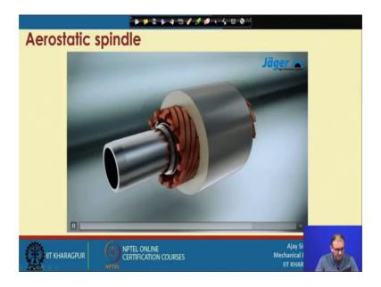
And this is the motor because we know that it is integral motor type of spindle you do not have a external motor and passing through the belt drive.
