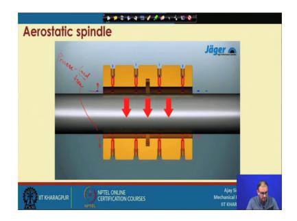
So, we know the pressure equal to load by area, so here area is reducing here at the time because of that what is happening the your pressure is increases this location when it is going down you can see that here area is increased. So, because of the higher area pressure equal to load by area correct. So, now, here area is this location area is high and this location area is less. So, because of that here the pressure now you have a large area.
