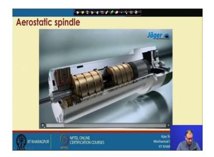
Now, you can say that you will note find any type of ball bearing or any other type of bearing because this bearing is a air bearing. So, instead of ball another thing that you will get some passages here. So, through with this whatever air is coming into the system that air will actually passed through this particular sockets or passages and then it will actually create a uniform pressure around the shaft right, so this is the passage for air.
