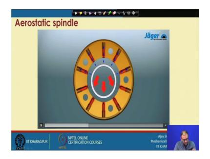
Your pressure will be different here, so on the upper of there is a low pressure and lower up there is a high pressure. So, whatever this red colour syringe or the nozzles are showing this will create more amount of pressure here and here this blue colour has the less pressure. So, because of this pressure difference again you particular shaft will again be in the centre position. So, that you can avoid this particular pressure difference correct.
