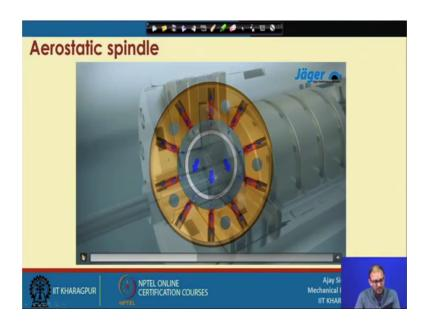
So, this is the way actually you will get the radial stiffness, and we know that this radial stiffness is very important when you do the milling operation.
