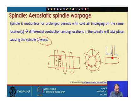
That when the spindle is motion less for a problem period with a cold air impinging onto the same location, so that is what is happening here. So, at that time what is happening the differential contraction among the location in the spindle will take place causing the spindle to warp. So, because of that we know that this is the one we are let us talk about the single only.
