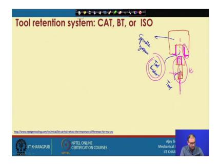
Now, coming to the tool retention system now what is the tool retention system; that means, once you hold this particular part now we know that we have all the thing that is bearing is also there right. So, this is the system and this is the tool holder and this is our tool correct. So, now, there are three location where we need a joint right.
