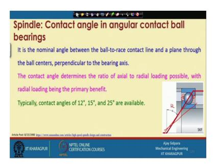
So, what is the contact angle here, so it is a nominal angle between the ball to race contact, so where is the ball to race contact, so this is the ball to race contact correct. So, this is the ball to race contact line, so where ever this contact is there you have to draw one line in a. So, this is the line passing through the ball to race and a plan through the ball center.
