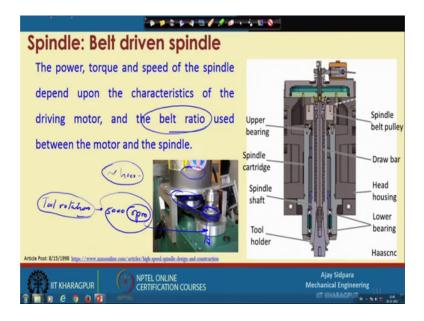
So, power torque and speed of the spindle depend upon the characteristics of the driven mo driving motor belt ratio used between the driven motor and the spindle, now you can see in this location here that this pulley is big and this pulley is small correct. So, now, when you are telling your tool that tool rotation, you are rotating at a 5000 rpm correct.
