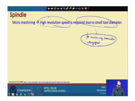
So, in micro machining spindle is very, very important high revolution speed is required to due to the small size of the diameter, that we have seen that we have to maintain the cutting speed correct. So, for maintaining the cutting speed is very important, so this is for maintaining reasonable cutting speed.
