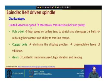
What are the disadvantage this is limited by the speed because it is a mechanical transmission belt and the pulley type of thing? So, if you increase the speed beyond a certain limit what is going to happen there is a slippage between the belt and the pulley and you are not able to transmit the full power of the spindle from one location to another location, pulley v belt type if you are using this belt type high speed on the pulley tend to stretch and disengage the belts.
