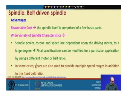
Let see what are the advantage because cost is reasonable that is obvious because spindle itself as a compre is comprised of a very few basic parts, wide variety of spindle characteristics available because that a spindle power torque spindle speed at depended on the driving motor to a large degree. So, you have a large variety of the driving motor, so that is not a issue final specifications can be modified for a particular application by using a different motor of the belt ratio.
