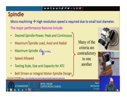
Yeah, so what are the measure performance features available or required for spindle is first is the desired spindle power the what is the power of the spindle, because that will decide that how much day for that you can get the how much force it will actually sustain during the machining peak power and the continuous. So, that is that continuous and when you have machining with a 40000 rpm or something how long you can continue with these things because there are limit on that also.
