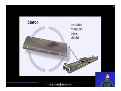
Correct. So, this is the stator. So, it includes magnet base and the shield because we have seen that we have un-wrapping that conventional motor stator and then it was becoming
