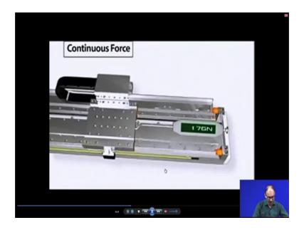
As on stator is the continuous force? Because now if you apply a force here, so how much is the force when you apply continuous current how much is the force you can get when you are moving this particular platform? So that is called forcer.
