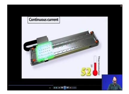
So, it is a continuous current. So, we have to apply the continuous current. So, that you can get this particular moment possible and we know that if you increase the current what is going to happen that we have a temperature rises so, with a (Refer Time: 11:10) and so we have to maintain that how much is the continuous current we can provide. So, that your whole system will work within the desired or the limited temperature zone.
