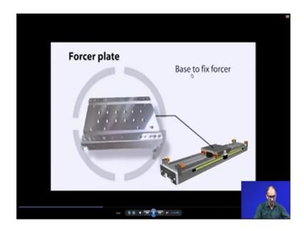
And this is a forcer plate on the top of that. So, it is base to fix the forcer and after that you put something on the top.
