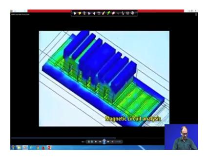
So, this is all the things about the magnetic circuit. So, let us not discuss this thing more right now. Because these things are used for the simulation and analysis before design purpose only. So, this is all about the umm linear motor. Right?
