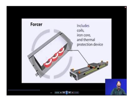
So, this is the complete assembly. So, forcer includes, so this is called forcer this part. So, it includes coil because you have to create a electrical signal here. Iron core is there because it is something like electro magnet kind of things and thermal and protection devices because you have to isolate this thing from the electrical problems
