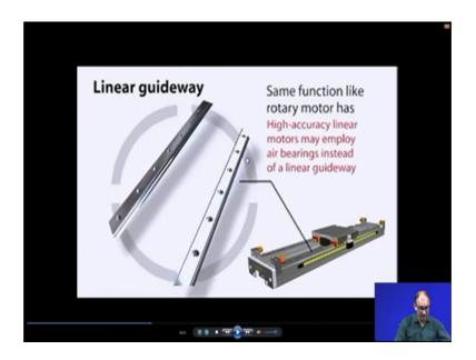
So, these are the linear guidesway. So, it is same function as the rotary motor has the right accuracy linear motor may employ air bearing instead of a linear guideway. So, here we have a different different option before earlier lecture we have seen that we have a linear guidesway, where we are using a different different kind of bearing hydrostatic bearing, air bearing. So, we can use air bearing here. So that you can even get very very
