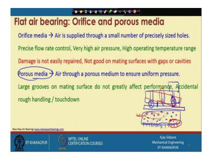
Another one is the porous media. So, now, what is going to happen that instead of those type of holes right. So, earlier we have seen that. These are the orifice now, instead of orifice, what we are doing? We are using one type of porous media. So, there are different small-small holes available, was some type of passage available. So, it is considered porous material right. So, what is going the air through a porous medium to ensure the uniform pressure?
