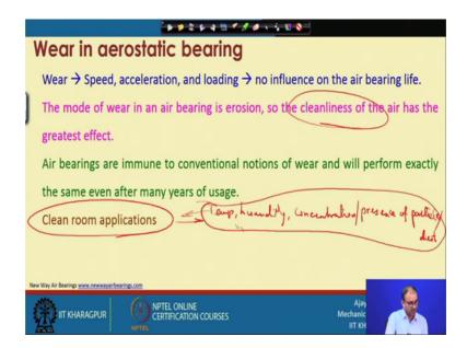
What about the wear, because wear has directly connection with the speed acceleration and loading right, if you increase the speed, your wear rate is high, if you increase acceleration, your wear rate is high. And if you increase your loading again, your wear rate is high, if there is a direct or the physical contact with the surfaces.
