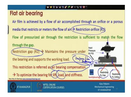
It maintains the pressure under the bearing and support the working load. So, we have to thinks that how much your pressurizing or we, how much we are supplying that is through the orifice that is applying and; that means, how much we are leaving it away. So, that is called the gap restriction, if the gap is more, what is going to happen that your gap restriction; that means, pressure will be very less here, because now area is increased.
