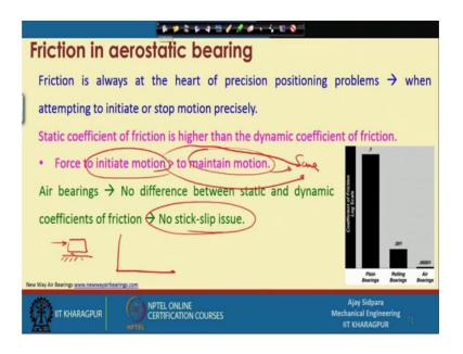
You can easily start the component, because now, we know that there is nothing in between these two only, air is flowing. So, your force to initiate the motion and maintain the motion both are same right.
