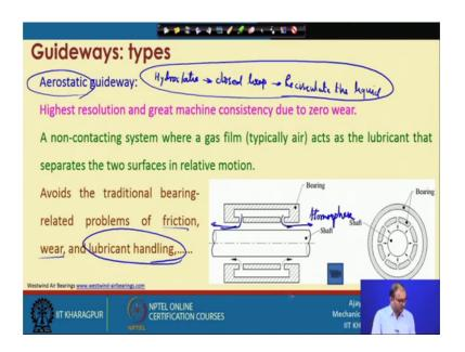
The traditional bearing related problems of the friction wear and lubrication handling, if you see that earlier case that where we are using hydrostatic part. There was one particular things, you might have noticed that it was a close loop system right. So, it is a hydrostatic, hydrostatic is a closed loop. So that means, that you have to recirculate the liquid correct; that means that here what we are doing that, we are actually not worried
