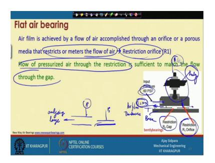
So, this is a flat air bearing type of thing. So, here what is the thing here? So, these are the two ways. So, it is mostly done by the orifice type of or the porous media that restrict the meter or meter, the flow of the air and there is called restriction orifice. Now, what is this restriction orifice that you have? You can see here that there are two things, a restriction orifice R 1 and restriction gape that is R 2 and now, you are providing the air
