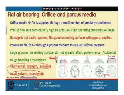
Now, you can see, this is the profile of the pressure. So, this is the pressure right. So, this is the orifice type and we are putting over orifice only. Now, if you can see that this orifice are matching with this particular peak pressure, you can see the, there is no material available. There no space available, nothing is available. So, you are getting a variation in this particular part.
