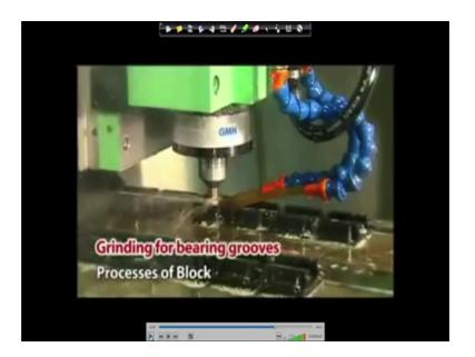
Because, earlier what we have discussed, it is for the single component, but if you have two component, which are coming into contact with each other, then you to create a reference surface for the another one also, after that operation you have to grind the bearing groove also, because you have to make sure, there is no any type of dimensional, problem torrents and should be as tight as possible, so that you will able any problem, at the latest stage.
