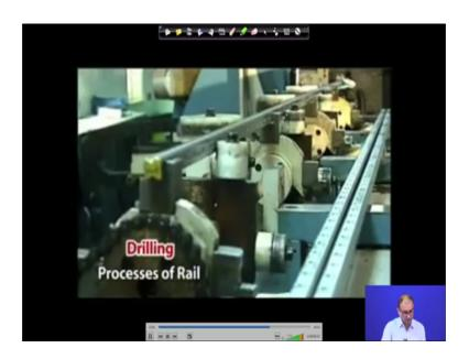
So, these are the straightening, first straightening, because initial you to straighten it and then you have to do drilling, because we have to mount many things here.
