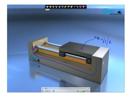
So, what is this thing that here, what we are doing that, this is a table and on the top of these, this is the slide. So, you consider a x or y, or it is mounted in vertical side, then it is a z axis right. So, we need a frictionless, this particular part. So, how this thing will work here?.
