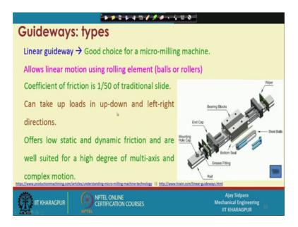
So, we have seen the, all the thing that these are the different components and how this is better than the other kind of things, linear guideway after the, that is called hydrostatic guideway.
