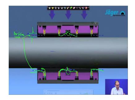
So, now, this is the interface. So, this is the shaft and this is the bearing and in between, this is the fluid filled. This is called air film and that is the same way, in this direction also correct, because we have to keep in this shaft, in the central position of this particular part. So, air is supplying from this part also, this is also and this way also.
