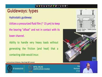
So, what are the advantage. It has ability to handle very heavy loads without generating friction heat, that are contacting slide would incur. So, in this particular, it will because now, we are using a liquid here. So, it will, it load, carrying capacity is very-very high in this case.
