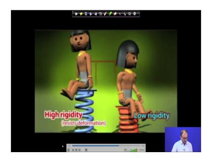
So, when you defined rigidity, a higher rigidity means less deformation or it will resist more deformation. So, this spring is not compressed more. So, it has a high rigidity and this one has a low rigidity, because it has compressed little bit more. So, why this thing is important? Because these things are important, when you are machining at a cutting tool, because when the cutting tool (Refer Time: 06:46), cut in contact with the workpiece tool, at that time there are force is occurs.
