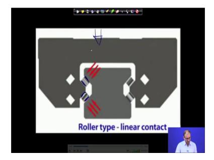
And now if you use a roller bearing then again it is the same thing here, but now you have a more contact jump points are here. So, it is a line contact now, because of the line contact your load caring capacity increases. Now you can add little bit high amount of load for machining or the doing a little bit aggressive machining at the micro machining center correct.
