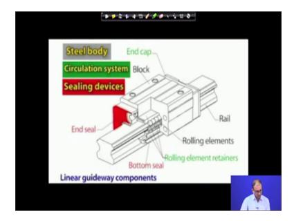
So, what are the components of this linear guides way. So, one is the steel body that is required, because on the top of that what we are doing we are mounting our work piece. So, that it can move in the x and y directions; that is the first component steel body.
