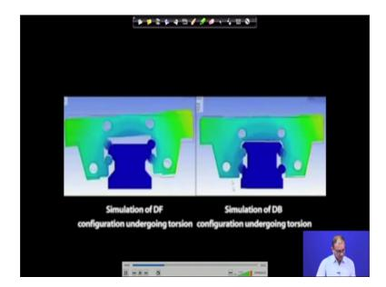
Torsion means; that means, you are moving in this particular direction and this is the same thing for the configuration undergoing the torsion; that is called DB type and this is called DF type. Now if you see this thing is moving little bit more in that particular sense, because now it is not able to resist that particular torsion motion comparative to this particular DB configuration.
