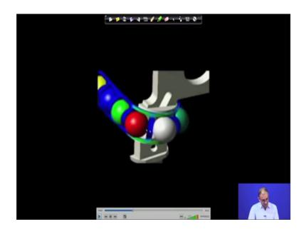
So, once you get this end block at that time, it will it will circulate from this to this only, it will not create any additional motion. So, these are the things. So, it will move in a particular confined motion only correct. So, this is the way this particular ball will move in the direction and this is the rolling element retainers. So, retainers are required, because these particular retainer will make sure that balls are not actually moving in a other direction.
