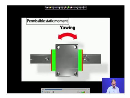
So, when you see from the top and that is called yaw motion that these things we have seen in that geometric error in the machining.
