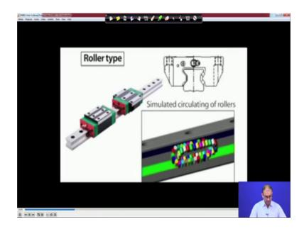
So, instead of balls what we are doing? We are using roller, so you get a like contact and you may get a more load caring capacity in this case.
