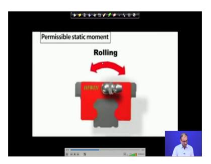
So, now these are the different different movements. Earlier it was load only, now it is a movement, so it is rolling movement. So, this is your vertical direction. So, it is moving on left and right at.
