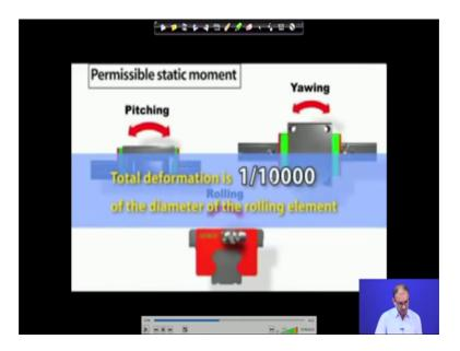
And this is called the pitch motion; that is looking from the left side or right side. So, these are the motions. There is mostly happens when you doing machining of the side cutting or something slot cutting, something like that. So, if under these condition also same thing the deformation is 1 of the 10,000s of the diameter of the rolling element.
