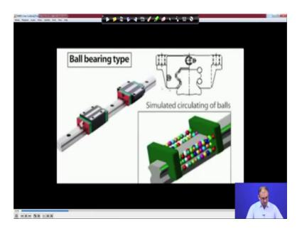
So, this is use for the ball bearing. So, now, if you are using a ball bearing then this particular motion will be something like this and other thing is a roller bearing.
