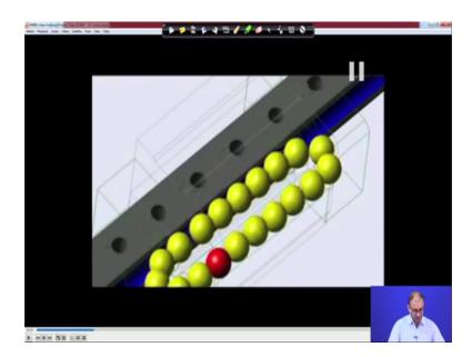
How this will work? You constraint the motions of the balls in such way that it will circulate continuously, when there is a motion between the drill and this particular ball.
