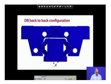
So, now this is called back to back configuration DB type. So, here now these particular balls have contact point; that means, center line moving in these particular direction that is called back to back configuration. So, its contact is outside of that part. So, what is thing this is simulation of DF configuration under the torsion part
