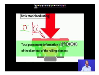
So, this is what it is, it should not deform permanently and so that is whatever load is happening, that is the load bearing capacity. So, total deform permanent deformation is 1 of 10000 of the diameter of the rolling element. Why we consider this rolling element
