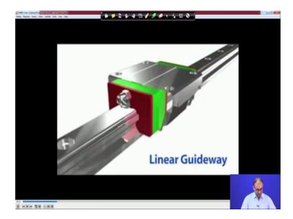
So, final solution is that instead of using a cylindrical shaft you actually go with the linear guide way. So, this is the guide way on which you mount all that subassembly like balls or rollers or different type of constraint motions. So, this is the advantage of that part.
