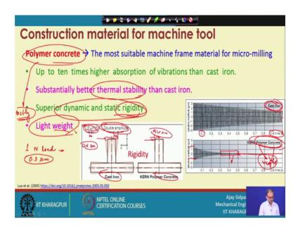
So, this is the way you can make the polymer concrete. So, polymer concrete is the most suitable of machine frame material for the micro milling process. So, why it is so, let us see the, so it is up to 10 times higher absorption of vibrations then the cast iron. So, this is one of the example, so of kern machine. So, that machine we will see the demonstration some time later.
