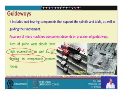
Now, coming to the guide ways; so now, what are the guide ways? So, guide ways; that means, on which you are putting all the components. If you are using a spindle then the on the spindle you are putting these guide way, because you have to move z axis in this direction. So, this will be the z axis when you are mounting vertical and if it is in a x y
