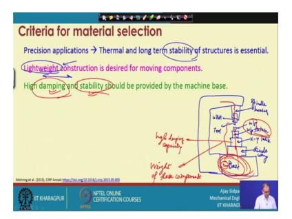
Suppose, first thing is the precision application. Suppose, your requirement is the precision, application then what we have to see that, we have to see the thermal and long
