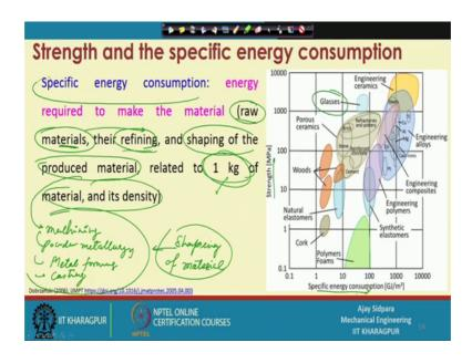
Another thing is strength and the specific energy consumption. So, this one more graphs. So, here different materials are given in the Y axis, it is a strength. So, this strength is increase, this is the specific energy consumption. So, what is this specific energy consumption, because if you see these materials that these materials not readily available; that means, wherever you are getting, you have to process this components.
