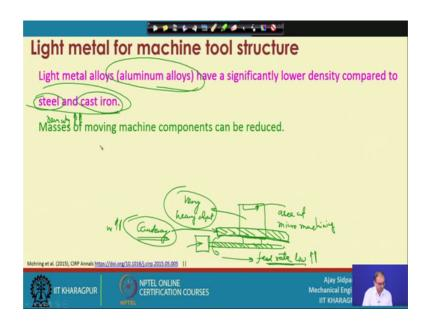
So, other than that whatever, we have seen that we can use, different type of metal, but there are light metals are also available mostly, it is a aluminum alloy or magnesium alloys. So, these materials have a significant lower density compare to the steel and cast iron, because we know for construction material mostly, we prefer for the base material, we prefer the cast iron and for other material. We prefer the steel, but the density is, density is high.
