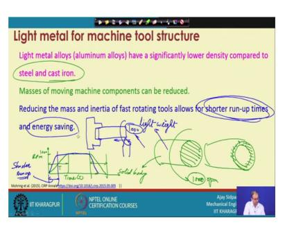
So, reducing the mass and inertia of fast rotating tools, allows the shorter run up time and energy saving. So, what does it mean that suppose, you have a solid body [body] and you want to rotate it, ok. So, when you rotate it, at the time what happens that you have now, suppose you, you are, you want to rotate it to the 1000 RPM ok. So, now, is a stationery
