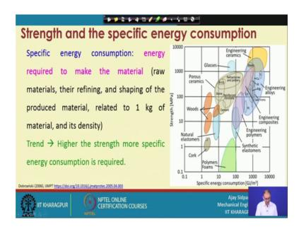
So, this is the trend; that means, if higher the strength or more the energy consumption is required that is, what is showing in this particular diagram. Just you draw these things, most of the things, it is balancing both the direction. So, this is the trend correct.
