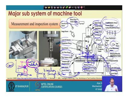
Now you can see here that how many different type of sensors you can put into the machining centre. So, this was from the very very old paper where it was means given in a very very generalised where what thing you can put into the machine. So, that your machine become very very intelligent now if you see the actual machining operation is here right. So, this is your cutting tool and this is your work piece right. So, this is a actual thing, but you can add many sensors here.
