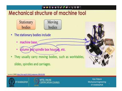
Now, what things are there there are 2 different compounds available one is a stationary body and this things are available. So, these are called stationary body that we have seen in the structure part that what was the machining stuff machine tool structure was there those was the stationary part and there are moving bodies available moving bodies are the x, y, z axes and the rotation around xyz axes and those things are moveable component.
