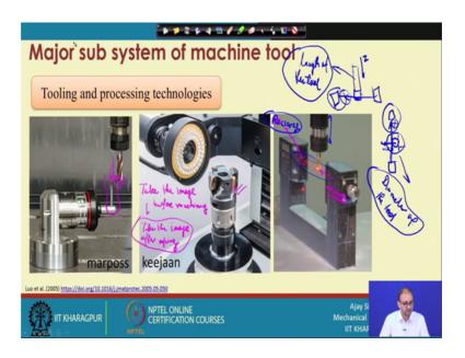
Then tooling and processing technology. So, till now what we have seen we have seen about the monitoring the machine tool operation in the machine itself. Now, tool is also important because we have to understand that how to monitor the status of the tool, when you are working with a micro tool or micro dimension we know it is a difficult to detect the tool we are and the tool breakage.
