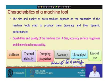
Throughput is also important that how many components you are getting that is called the production rate, rate of processing or we can say it the production rate correct. So, that is important, because even if everything is there, we should have reasonable amount of throughputs. So, that we can just justify the cost verses the production rate, because the cost of the machine is; obviously, very high.
