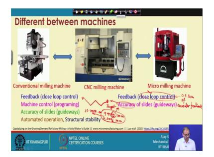
Now we understood the difference between the conventional milling machine and the CNC milling machine, but again there are some limitation of the CNC machine when you are working at a micro level, because there are many components which may not give a satisfactory results when you are working at a micron level, when you are working the tens of microns or hundreds of microns, sometimes this is also not enough.
