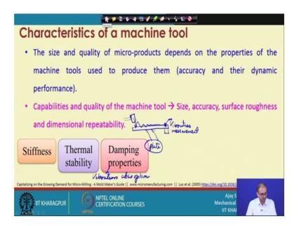
Damping properties; Damping property means the capacity of vibration absorption; that means, suppose you have one table here let us consider, and here you have sensor and you are hitting with a hammer at this location, you are hitting at this location.
