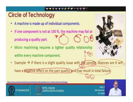
So, now, this is the example that we have discussed here, that if there is a slight quality issue with a spindle quality issue in the sense that it is either not rotating exactly as per the rpm, or it not aligned actually exactly at the centre. So, this is you consider the speed center in the z axis and this is you consider as the axis of your spindle, and then this is the angle theta; that means, your angle not matching exactly this part.
