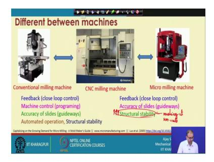
So, rigidity of or the structural loop stability should be extremely high in this particular case, and which is not the case of the first two. So, these should be very high and then only you can get the machining at micro scale.
