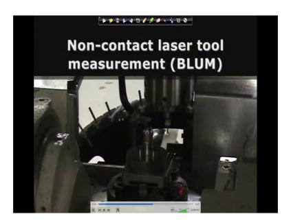
So, now, once the operation is over now, you have to confirm whether it has a required dimension machined or not. So, now, this is the non contact tool measurement sensor. So, this particular sensor will sense and it will measure the dimension of this particular machine or machine component and then once it is confirmed then only it will go to that particular part. So, that thing was done for measurement of the status of the cutting tool.
