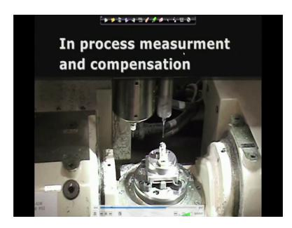
So, this is which is used for measurement of this particular component. Earlier one was used to measurement of the status of the cutting tool. So, it is a laser guided. So, this particular tool will move into that location and laser will confirm the edges and the length and this is used for measurement of the cutting.
