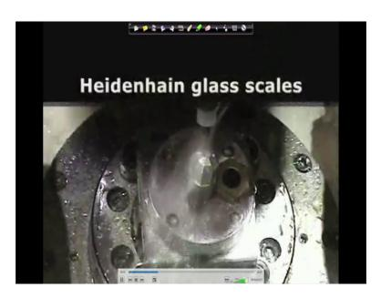
So, this is the true 5 axis. Now, this, whatever is rotation, this rotation is actually along the z axis, but it is inclines, so we are not looking at the z axis, but if it is exactly per perpendicular to this table perpendicular to z axis then you can see that this rotation is along the z axis. So, this is called c axis.
