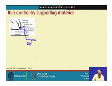
So, that is called the burr control by the supporting material. Because now we know that burr formation mostly occurs at the; this particular location. Hence at the edge of the parts this is the work piece edge, correct. So, when your tool is completely coming out of the workpiece you are this particular material will be actually located here in terms of the burr.
